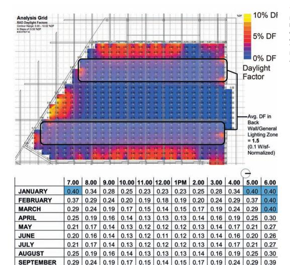
Daylight study showing estimated lighting use for each hour during each month in the highlighted daylight zones, in Watts/ft<sup>2</sup>. The upper graphic is an Autodesk Ecotect output of a Radiance analysis.
