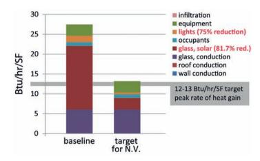
A lab building at the University of Washington used an eQuest energy model to simulate peak cooling load conditions. In order to eliminate a mechanical cooling system and use only natural ventilation for cooling, peaks loads needed to be reduced by 50% from a baseline. The project team was able to test many options, finding a balance that met the target by reducing glazing percentage, using windows with different properties, and providing shading during peak periods.
