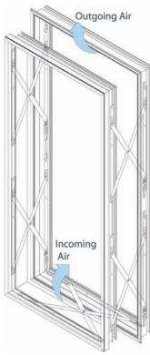
Photograph of the type of operable windows used at the Bullitt Center. Window diagram shows equal opening size around window's perimeter to reduce wear and provide even, controlled airflow.
