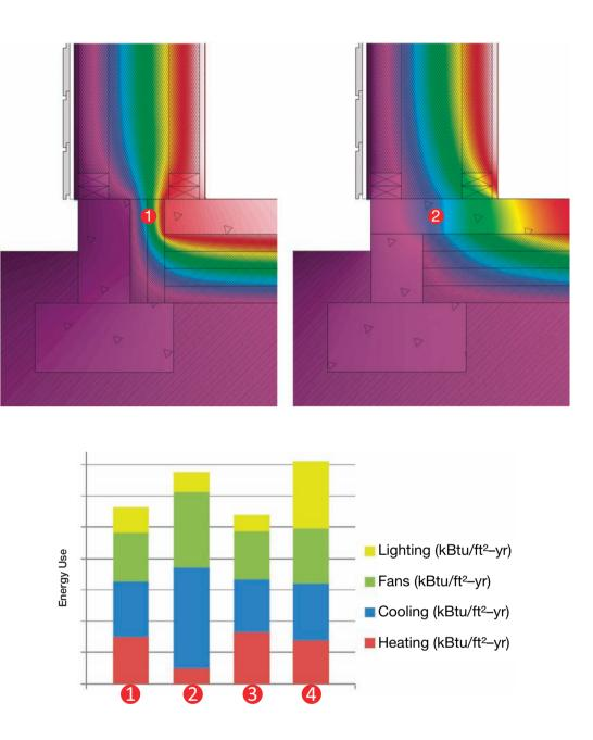
In many cases, thermal bridges occur due to a steel or concrete structure that spans from a conditioned space to an unconditioned space. This happens at cantilevered balconies, eaves, canopies, and in many conditions in most buildings. Metal framing studs also provide thermal bridges, reducing the thermal resistance of an insulated wall assembly by nearly half.
