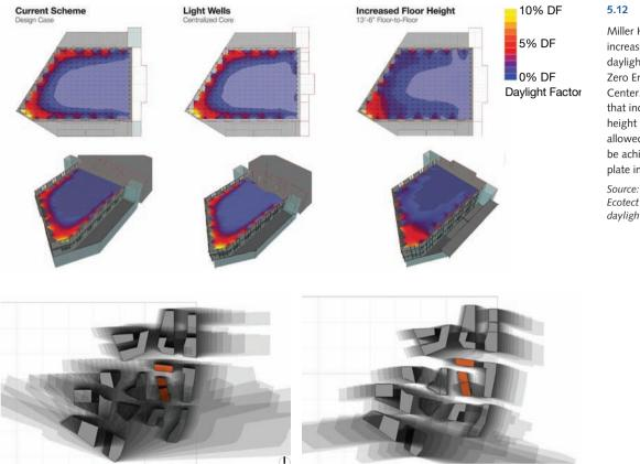
Miller Hull studied the effects of increasing floor-to-floor height on daylighting for the 6-story, Net Zero Energy targetted Bullitt Center. An early study showed that increasing the floor-to-floor height from 11'4" to 13'6" allowed successful daylighting to be achieved on 65% of the floor plate instead of only 23%.
