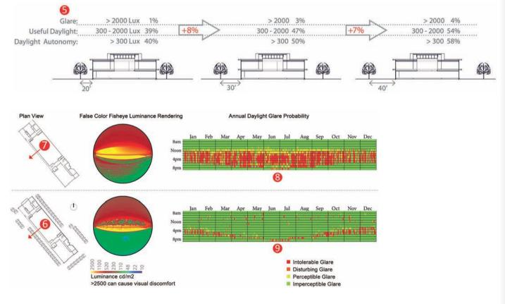
A baseline option (7) was run with no trees for comparison. The baseline option is exposed to intolerable glare throughout the afternoon all year (8) due to direct sun and high contrast in the field of view. The proposed option with trees successfully controls glare up until sunset with less direct sun and lower contrast in the field of view (9). This schedule can be fed into blinds schedules for annual lighting energy use estimation.
