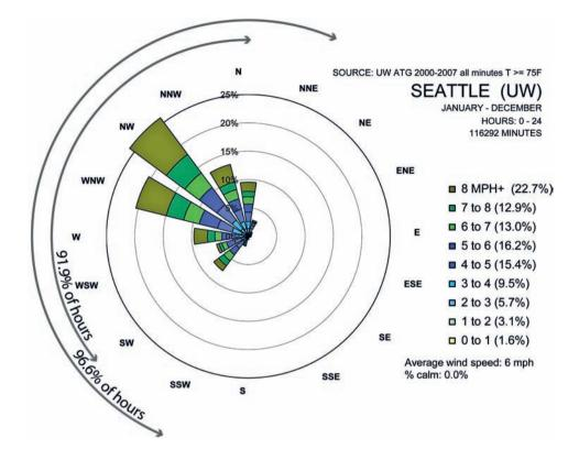
Local wind data has been compiled to show frequency, direction, and speed during those hours of the year where the outdoor air temperature is above 75°F. This data helped determine that wind direction and speed were consistent enough to provide natural ventilation cooling for the offices at the University of Washington Molecular Engineering & Sciences Facility.
