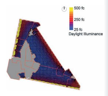
**10.50** Daylighting simulation, illuminance levels, Sept. 21 at 9 a.m.
