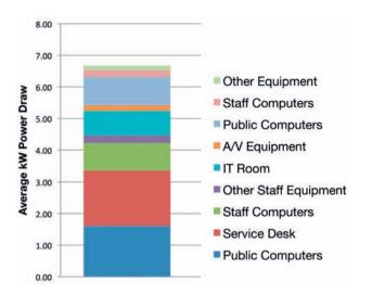
Plug load analysis for the West Berkeley Library was based on surveys of the existing library, and included over 90 individual plug loads. Since the project targeted Net Zero Energy and reduced all other loads, plug loads will account for around 40% of the project's energy use. The chart breaks down plug loads into attributable uses; computers make up most of this load.
