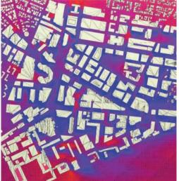
Completed wind speed studies were used to mass new structures to block undesirable winter winds through public plazas. This study was completed as part of the Cambridge Master Plan in Boston, using Autodesk Vasari 3D for a Computational Fluid Dynamics simulation, with false colors representing wind speed. Wind is simulated to come from the upper left.
