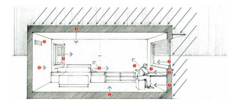
A single room showing some of the inputs into an energy modeling software to determine energy use and comfort (1–9).
