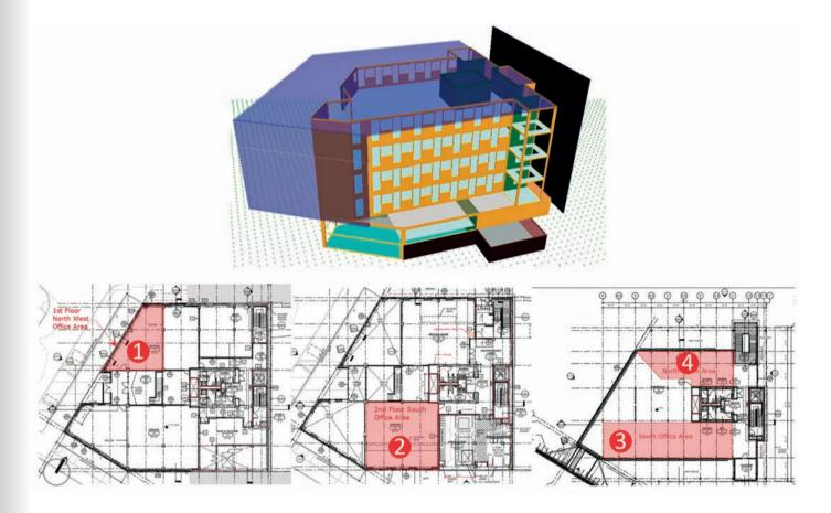
3D TAS model and selected indicator floor plans. While all zones were tested, the team focused on operative temperature in four indicator zones (colored red) in greater detail. The internal temperatures are shown on the chart with and without radiant cooling.
