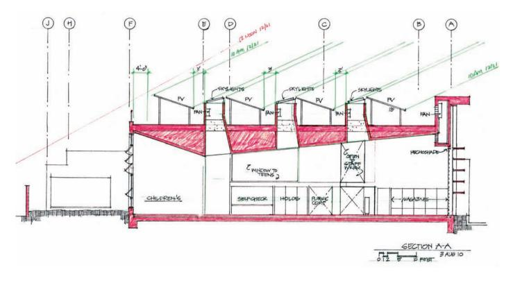
Early design section through the reading room of the Net Zero Energy-designed West Berkeley Library. The design team used a combination of intuition and design simulation to create a roof form that correctly balanced the space for renewable energy, deep light wells, and natural ventilation. See case studies 8.2 and 9.1.
