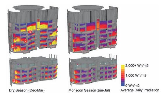
This project includes two residential towers and a number of villas. The towers each contain 2-story units at the upper floors over 1-story units. Residential balconies and the majority of the large glazed areas were oriented to the south to incorporate views and control solar gain. Metal mesh screens provide solar control for the limited openings on the east and west façades while allowing free airflow for cooling breezes. The north side has a balcony and operable glazing for cross-ventilation.
