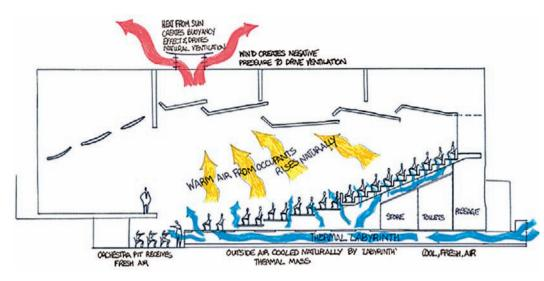
Concrete "earth tubes" beneath the seating use thermal mass and evaporative cooling to maintain comfort even during peak conditions. This system was proposed early in the design phase, chosen as a project goal, and successfully eliminated the cost and energy use associated with a mechanical cooling system.
