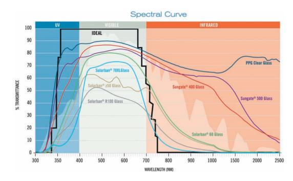
Spectrally selective coatings allow glazing products to reflect solar irradiation outside the visible spectrum without significantly reducing visible light transmittance. This allows low-SHGC products with high Tvis. Source: Courtesy of PPG Industries.
