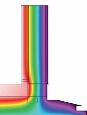
Calculation of thermal bridging effect on heat transfer.
