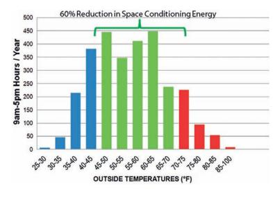
Temperature bin chart showing in green temperatures that require no mechanical heating or cooling.
