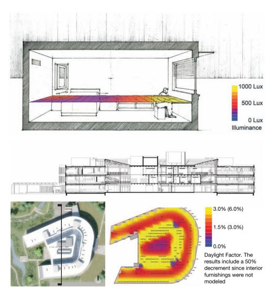
The daylight factor is independent of orientation and time of year, though it may take into account adjacent buildings and shading devices if the simulator chooses to include them. An office is considered well daylit with a DF between 2% and 5%.
