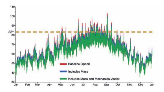
An energy model predicts hourly indoor temperatures based on three options. The third option lowers the indoor temperatures so that >97% of occupied hours (8 a.m.-8 p.m.) are below 83°F, allowing natural ventilation to provide a level of cooling acceptable to the client. See Case Study 9.1.
