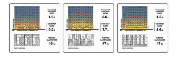
geometric aspects that define the daylight zone. For skylights, useful daylight will spread approximately half the ceiling height beyond the edge of the skylight in plan view.
