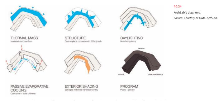
Simulation tools were used for a variety of purposes, from choosing the materials based on embodied energy and life cycle analysis, to shaping the building's daylighting, airflow, and energy use.
