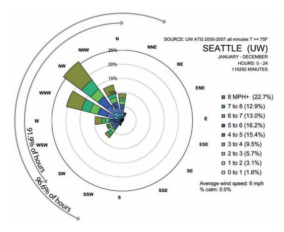
Wind rose for occupied hours where the outdoor temperature  $>75^{\circ}F$ .
