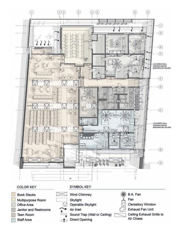
Floor plan showing layout of airflow systems.
