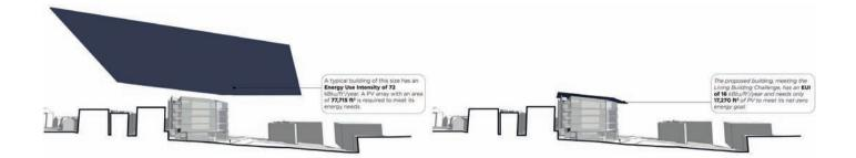
The left image shows a solar photovoltaic array extent required to meet the annual energy needs of a typical office building the same size as the Bullitt Center in Seattle. Using an integrated approach, asking the right questions, and evaluating decisions using experience and simulation, the array necessary to achieve Net Zero Energy was reduced to fit on site.
