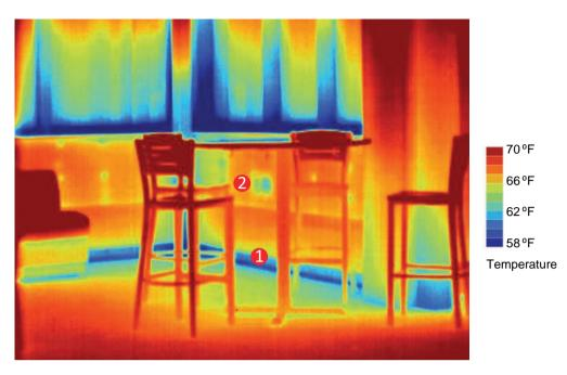
Thermal image showing the relative temperatures of interior surfaces. This type of image can be used to locate air leaks and thermal bridging. The connection between the wall and floor (1) allows a thermal bridge or air leakage from the outside. Air often leaks through the drywall penetration for the electrical box (2). The blue area at the base of the window shows cold air circulating due to conduction through the window, a typical occurrence.
