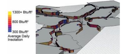
analysis was run to help determine which façades were most in need of shading, with the results being characterized as "average daily" irradiation to make the numbers more understandable.
