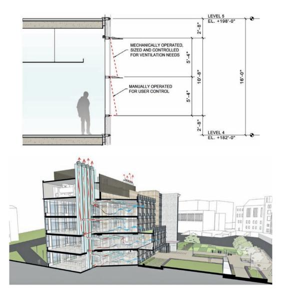
More detailed simulations were not necessary, as the stack exhausts incorporated a number of enhancements to airflow: "solar chimney" windows at the top of the stack super-heat the air which increases the airflow; turbine ventilators, which are driven by wind; and back-up electric motors to drive the turbines in case the airflow is not adequate.
