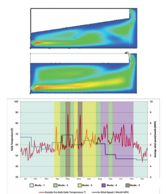
CFD studies to determine if a sloped or flat ceiling affects the cooling airflow near the floor level.
