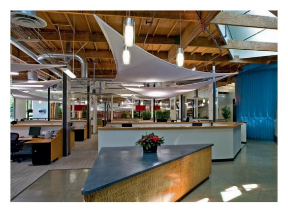
The Net Zero Energy offices for DPR Construction in San Diego, designed by Callison as part of an integrated project team, used simulation to inform strategies such as natural ventilation, daylighting with light tubes and light-diffusing tensile fabric, skylights, large fans to circulate air, and an advanced understanding of thermal comfort using the adaptive thermal comfort model.
