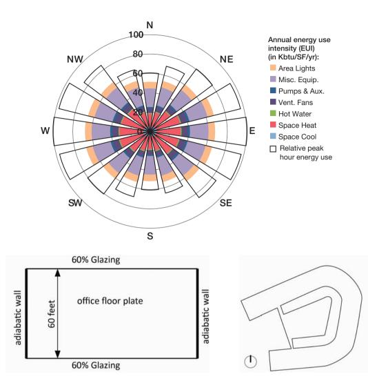
model was performed. The results generally indicated that a 60' width would be ideal to get a daylight factor of 2% throughout the majority of the floor plate with 8' of continuous glazing (from 2'6" sill to 10'6") on both sides.
