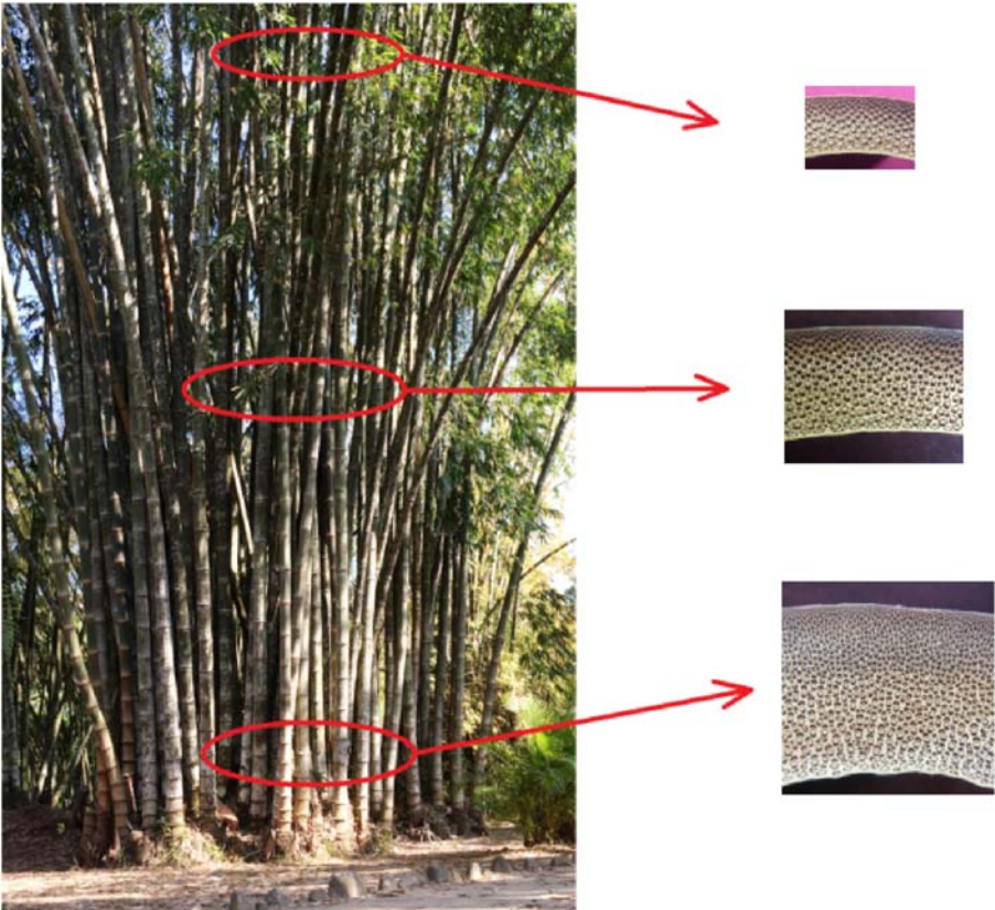
Figure 2.14 Original location of samples in the culm.
