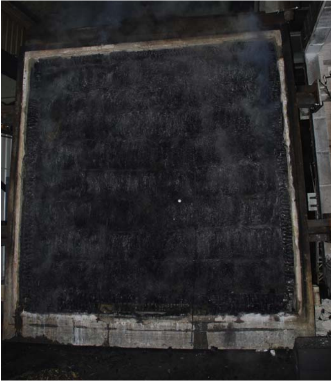
Figure 6.9 Straw bale panel after fire test.
