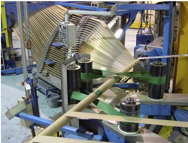
Figure 16.4 Paper tube manufacturing operation. With permission from Pakea.
