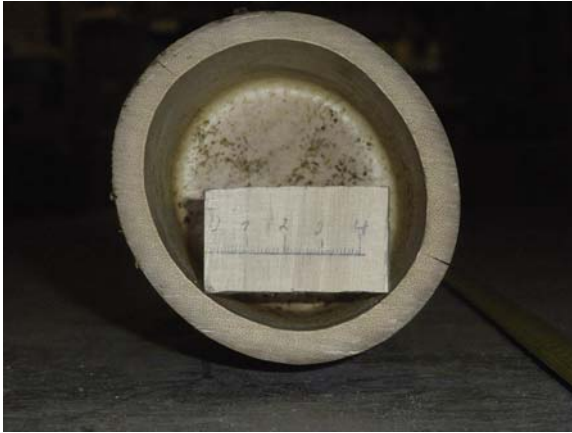
Figure 13.14 Bamboo rarely is absolutely round. Note also the fissures at the southeast quadrant and northwest quadrant (scale shown is in cm).
