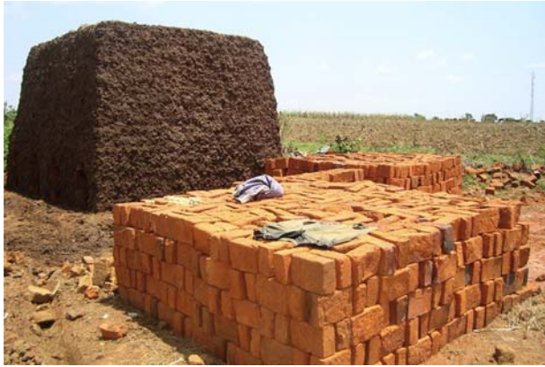
Figure 9.2 Small holder fired brick community project at Mumias in western Kenya. The absence of trees may be noted, most having been cut to provide energy for firing bricks. Courtesy of the author.
