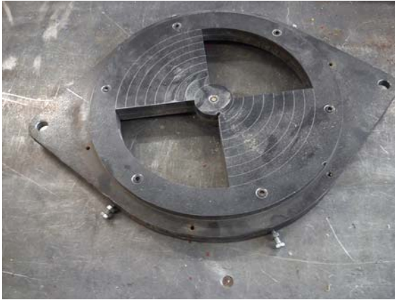
Figure 13.17 Bow-tie-shaped platens used in shear tests for bamboo. © David Trujillo.
