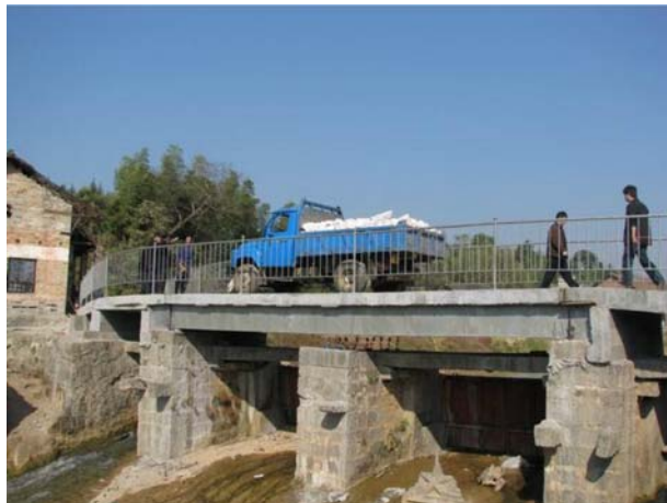
Figure 15.15 Glubam roadway bridge under truckload testing.
