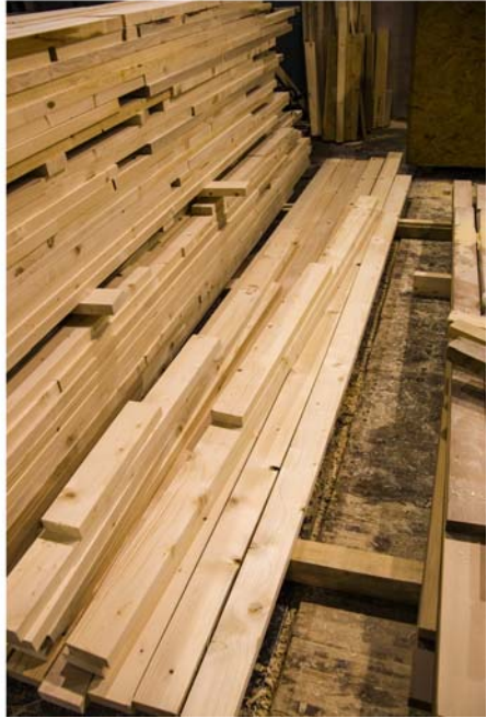
Figure 12.15 (a) CLT panel (five ply) and (b) CLT laminates prior to gluing.
