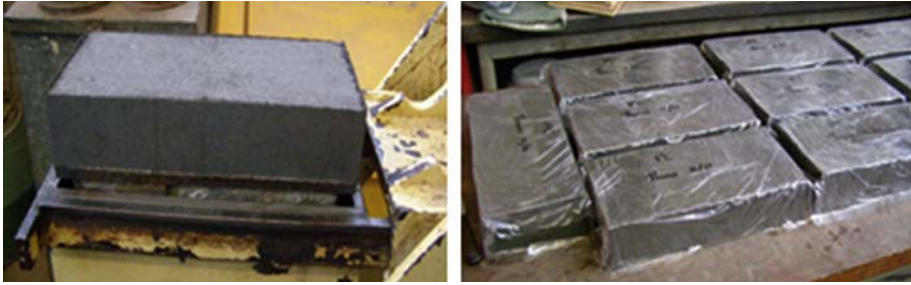
Figure 9.6 Clay–PFA ‘Eco-brick’ made sustainably by using the already proved sustainable lime–GGBS blended binder.
