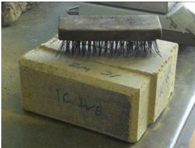
Figure 8.35 Oven-dried block and wire bristle brush.
