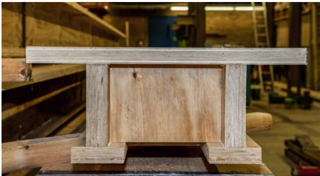
Figure 12.13 LVL composite beam with plywood gussets.
