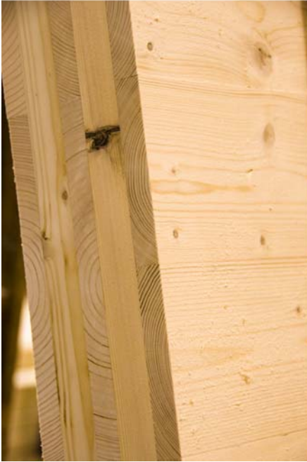
Figure 12.15 (a) CLT panel (five ply) and (b) CLT laminates prior to gluing.
