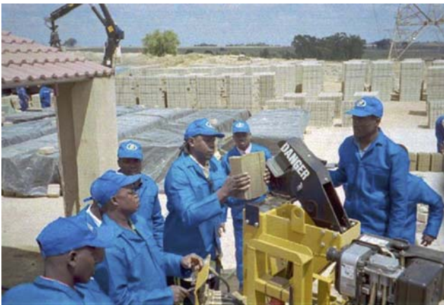
Figure 8.12 Handling and temporary stacking of freshly produced block. African Standards Organisation, 1996. Standards on CEB Construction: Compressed Earth Block Masonry ARS 670: Part 4: Code of Practice for Production and Construction.
