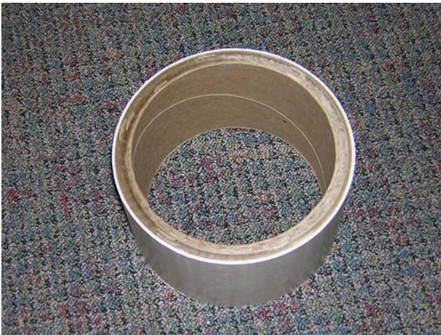
Figure 16.13 A 160-mm-ID, 16-mm-thick paper tube with an overmolded 3-mm pultruded outer layer.
