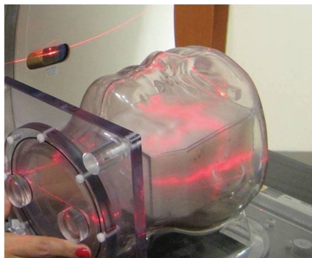
Fig. 50.3 RPC Head and Neck phantom. Positioning the RPC head and neck phantom for imaging, in preparation for treatment planning and treatment
