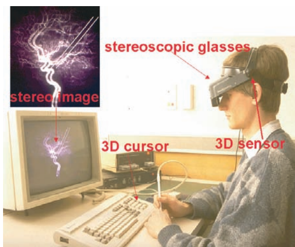
Figure 8.29 True 3D visualization obtained with stereoscopic glasses and a 3D head sensor to evoke head movement parallax. A 3D cursor allows the viewer to navigate the probe naturally through the blood vessel tree. (Development of Lab. Medical Image Computing, 1989).
