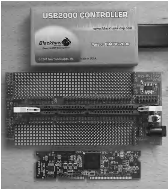
Fig. 3.73 System for developing software and hardware: F28335 control card, CC28xxx docking station and USB2000 Controller
