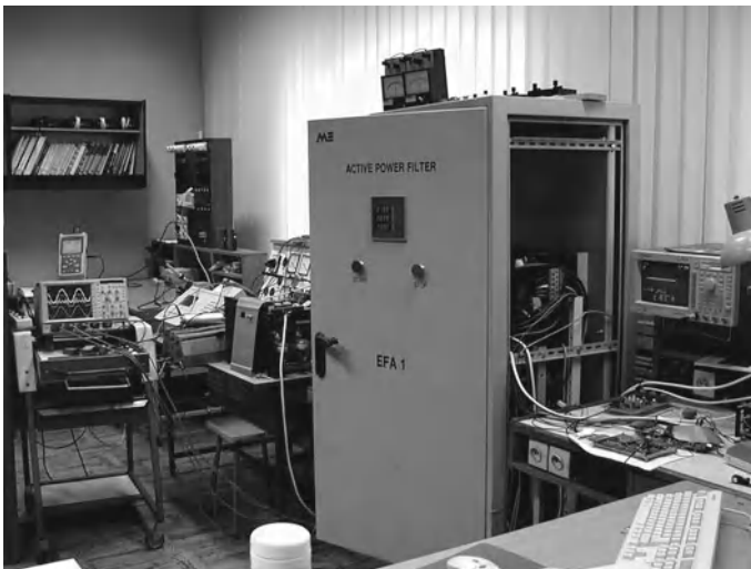
Fig. 4.23 Shunt APF at the UZ laboratory
