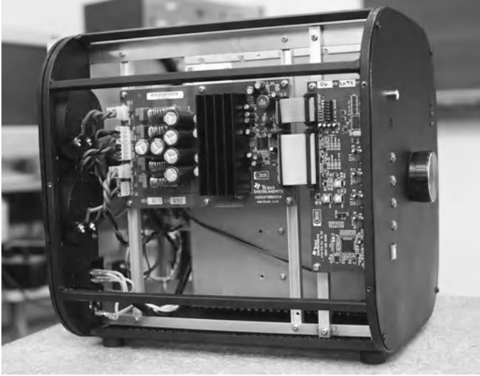
Fig. 5.19 The 2 × 316 W digital stereo amplifier with the hybrid supply unit
