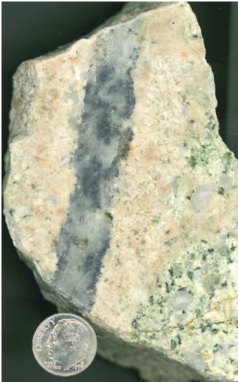
Figure 2 Vein of quartz-molybdenite ( \text{MoS}_2 , grey) ore surrounded by alteration envelope of pink alkali feldspar in polished slab of altered porphyry granitoid, Nevada Moly (Hall) mine, near Tonopah, Nevada. US 10cent coin for scale.
