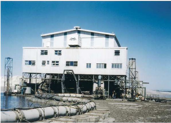
Figure 8 A dredge working on a deposit of rutile and zircon on Stradbroke Island off the Queensland coast. Such large and complex installations require capitalization running into millions of dollars. Photograph by GJH McCall.
