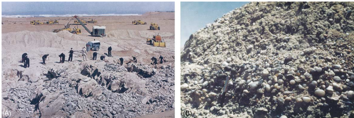
Figure 5 Diamond deposits on the south-western coast of Africa. (A) Diamonds are concentrated in deeply gullied wave-cut rock platforms exposed after stripping off later wind-blown sand cover. (B) Well-rounded hard pebbly gravel exposed on a raised beach. The heavy mineral content includes diamonds in hydraulic balance with larger pebbles. (Fountain pen lower left shows scale). Photo: GR Davis.
