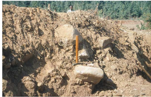
Figure 3 Colluvial boulders of kyanite being mined at Lapsa Buru, India. Kyanite ( \text{Al}_2\text{SiO}_5 ) is an industrial mineral used in mullite refractories such as sparking plugs. Photo: GR Davis.
