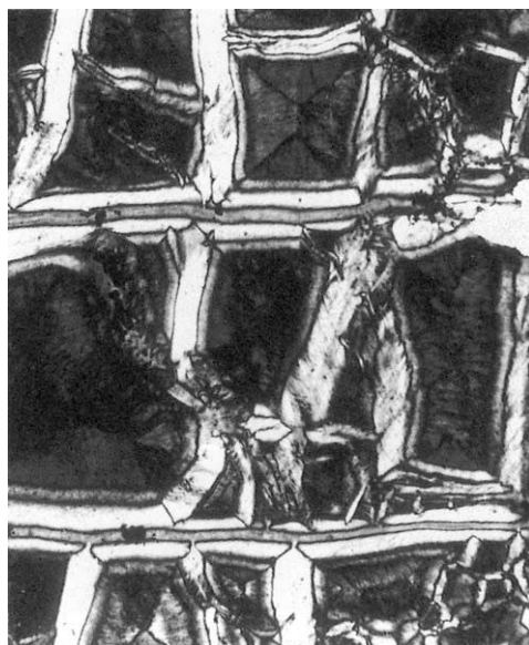
Figure 8 'Window' and 'hour-glass' textures of chrysotile and lizardite in serpentinite. Crossed polars \times 120 .
