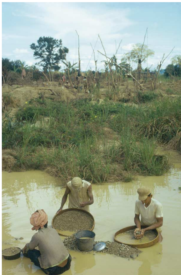
Figure 3 Washing gemstone concentrate in a small pond (Pailin, Cambodia). © Alan Jobbins.
