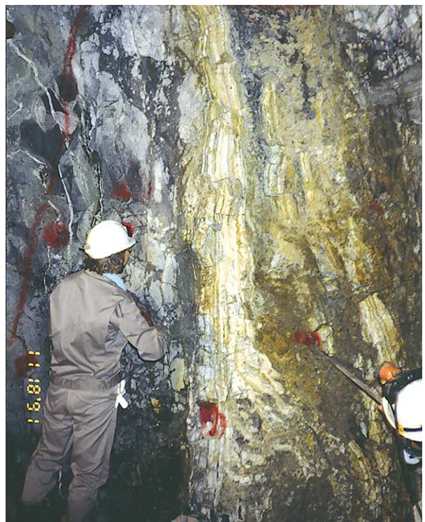
Figure 4 Banded crustiform epithermal veins of quartz in brecciated rock comprise the main ore type at the underground Hishikari Mine in Japan, one of the world's richest gold mines.
