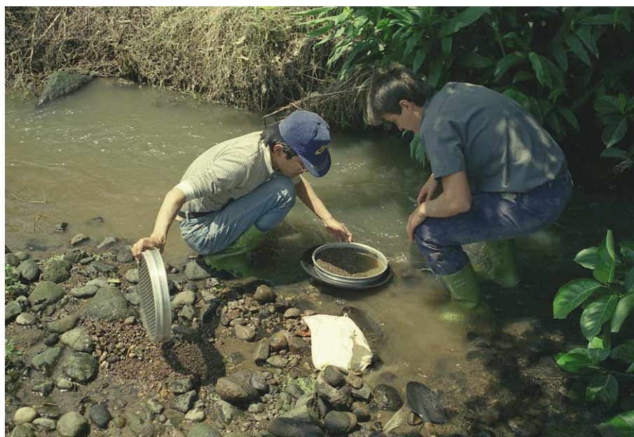
Figure 3 Geochemical sampling in eastern Taiwan. Sediments are dug from the creek bed, sieved to remove the largest pieces, and the finer fraction is bagged and sent to a laboratory for chemical analysis.
