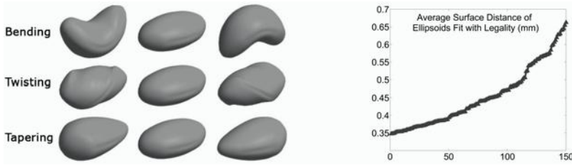
Fig. 3. Left: warped ellipsoids by three deformations of bending, twisting and tapering. Each deformation is shown as -2\lambda/0/+2\lambda away from the mean; Right: fitting results of 150 sample images shown as the average surface distances from model to binary boundary.
