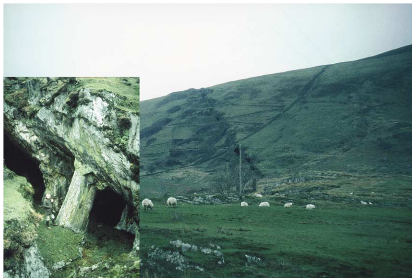
Figure 1 Ordovician ironstones, Betws Garmon, North Wales, UK (inset showing the steeply inclined stope method of underground mining for the deposit and a residual pillar of magnetite-rich material).
