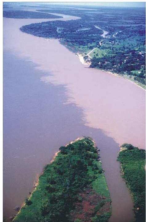
Figure 9 Large-scale Kelvin-Helmholtz instabilities generated along the mixing layer between the Rio Paraná (left, clearer water) and Rio Paraguay (right, higher sediment concentration), Argentina. Flow is away from the viewer, and the width of the image is approximately 1.5 km.
