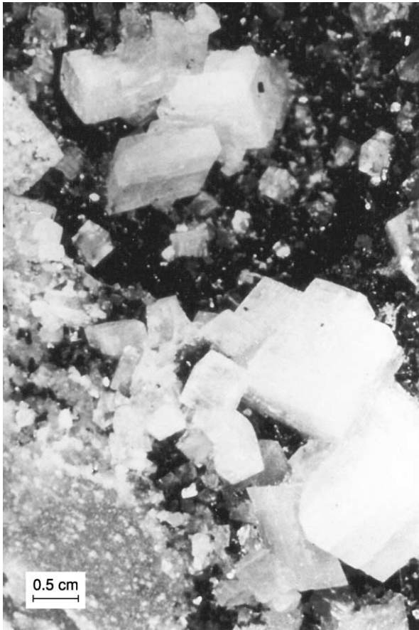
Figure 11 Core specimen of milky-white saddle dolomite cement in a vug that is coated with solid bitumen ('dead oil'). Host rock is grey matrix dolomite. Saddle dolomite appears as a large crystal in the centre and lower right, with undulous extinction. From the Devonian Nisku Formation, Alberta, Canada.
