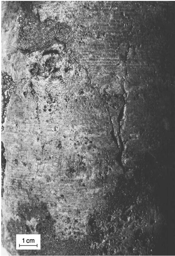
Figure 7 Dolostones consisting of domains of relatively tight, light to medium grey dolomite intergrown with domains of highly porous, brownish dolomite. From the Devonian Nisku Formation, Alberta, Canada.
