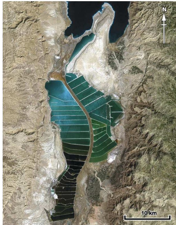
Figure 7 Satellite image of the salt pans at the southern end of the Dead Sea. The very saline waters of this lake are directed into shallow pans and evaporated to extract salts rich in bromine. This is a LANDSAT-7 ETM image using bands 3, 2, and 1 for red, green, and blue colour channels.
