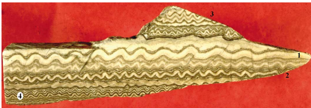
Figure 12 Harmonic and disharmonic folding in a specimen of the Castile and Todilto evaporites, New Mexico, USA (c.f. layers 1 and 2). Some of the folding (layers 1 and 2), can be described by the theory of single layer buckling, some by the theory of multilayer buckling, (3) and some (4) by the theory of buckling of an anisotropic material.
