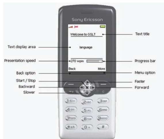
Figure 8. Button assignments for RSVP on a Sony Ericsson T610 mobile phone
