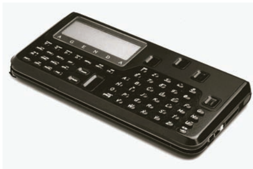
Figure 4. Sample chord keyboards (Douglas Engelbart and Microwriter Agenda)
