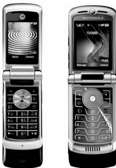
Figure 18. Keypads of the Motorola K1 and V3xx phones (showing the abstract-with-one-example design). Both images © 2007, Motorola, Inc. Reproduced with Permission from Motorola, Inc.
