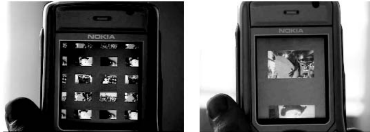
Figure 7. Picture browser application; the application automatically adjusts the zoom level to help the user browse
