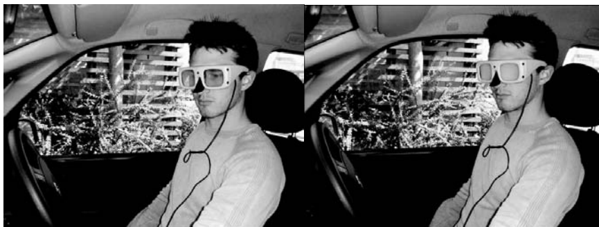
Figure 4. The occlusion method with participant wearing occlusion goggles, with shutters open (left) and closed (right)
