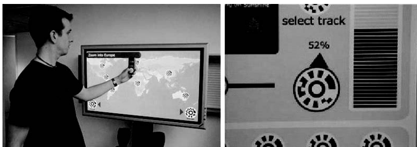
Figure 3. Using the phone to manipulate tagged widgets such as buttons, dials, and sliders (Madhavapeddy et al., 2004). Reprinted with permission from the authors.
