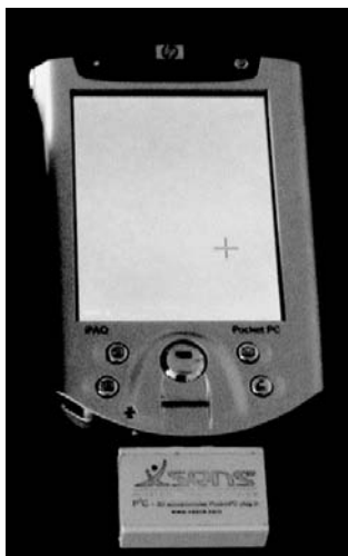
Figure 4. PDA with the Xsens P3C accelerometer attached to the serial port
