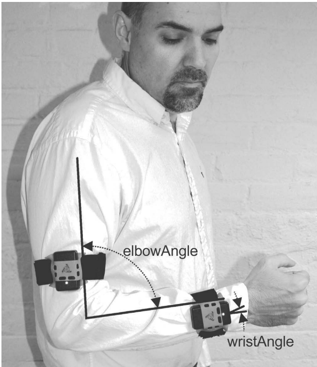
Figure 20.7: Sensor placement for joint angle measurement.
