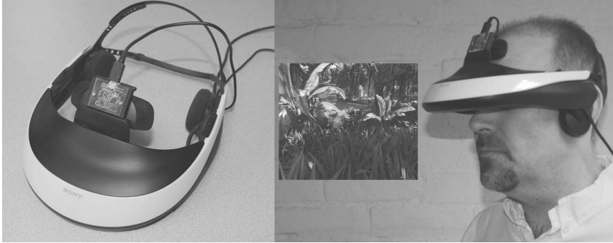
Figure 20.5: YEI 3-Space Sensor for head tracking on a Sony HMZT1 HMD.
