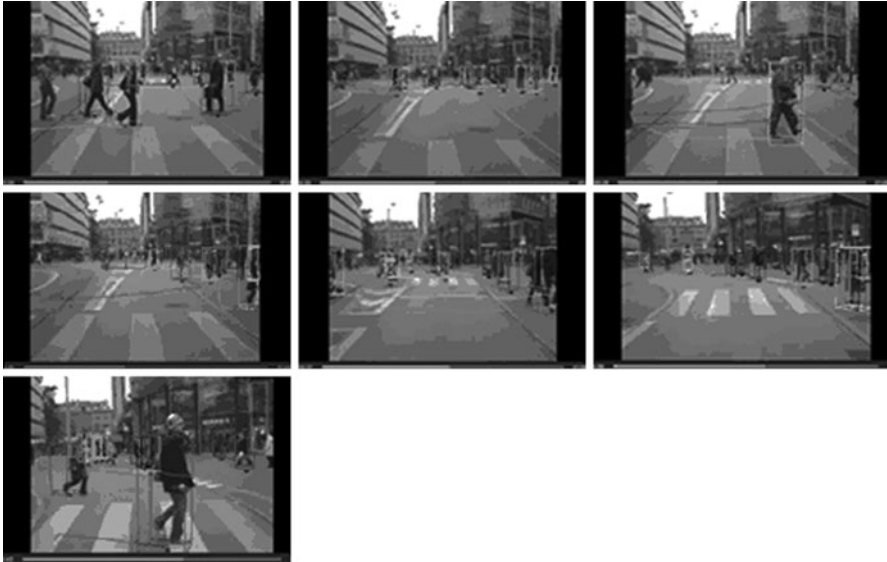
Fig. 21 Image taken from the paper Coupled Object Detection and Tracking from Static Camera and Moving Vehicles by Bastian Leibe, Konrad Schindler, Nico Cornelis and Luc Van Gool / Screenshots showing the tracking of pedestrians. 3D localization and tracking results from inside a moving vehicle. ( http://www.vision.ee.ethz.ch/~bleibe/papers/leibe-detectiontracking-pami08final.pdf )
