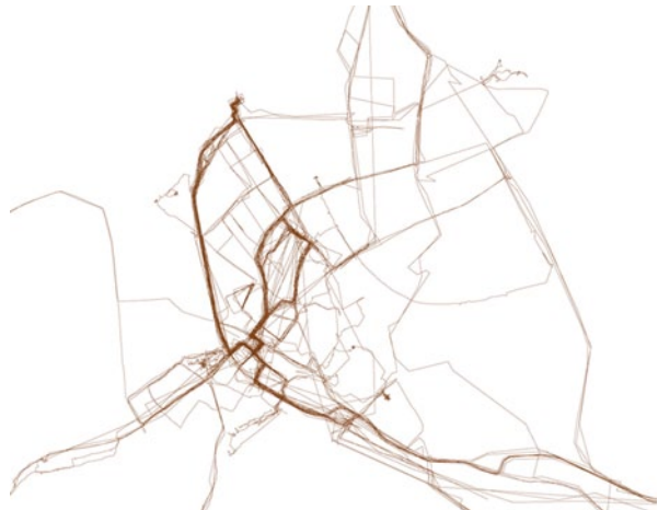
Fig. 2 Image by urbanTick / the straight lines occur where the GPS device had a weak satellite signal or lost the connection
