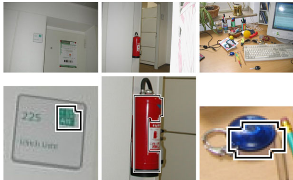
Fig. 4.18 Top : some training images with targets (name plate, fire extinguisher, key fob). Bottom : The part of the image that was marked for learning (region of interest (ROI)) and the contour of the region that was extracted for learning (most salient region (MSR)) (images from [5])
