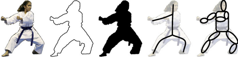
Fig. 3.2 Spatial shape (posture) representations. From left to right: performer template, bounding contour, silhouette, skeletal, parts representations
