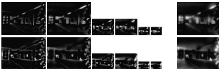
Fig. 4.8 Left : the 12 intensity scale maps I''_{i,s,\sigma} . First row : the on-maps . Second row : the off-maps . Right : the two intensity feature maps I'_{(\text{on})} and I'_{(\text{off})} resulting from the sum of the corresponding six scale maps on the left
