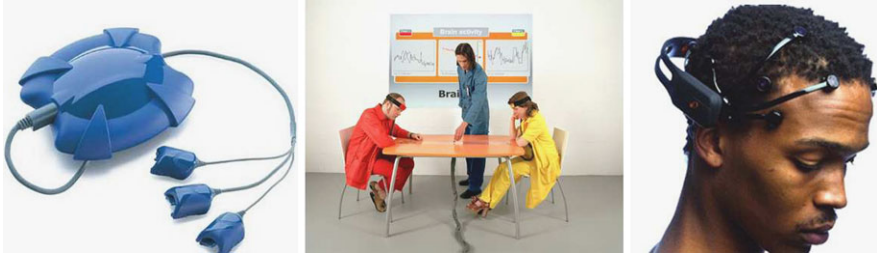
Fig. 14.5 Different physiological input devices: the Wild Divine (2001) [31] USB biofeedback hardware; the Brainball (2000) [10] EEG installation; and the Emotiv (2010) [19] wireless headset with advanced EEG measurements
