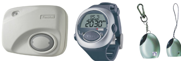
Fig. 12.4 Three commercial wearable devices. From left to right: Fall detector (detecting relative angle), elopement detector (based on radio frequency), elopement detector (based on infrared sensing)
