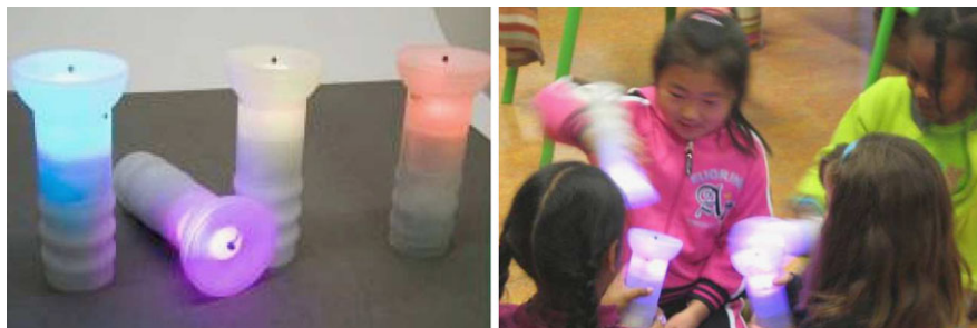
Fig. 14.8 ColourFlares [8], interactive objects that elicit open-ended playful interaction by changing colors when they are rolled and shaken
