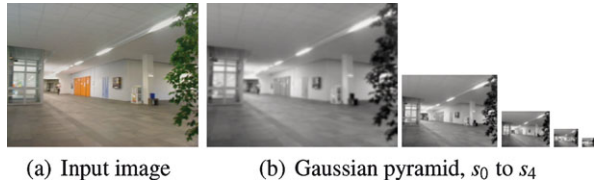
Fig. 4.6 (a) The image which serves as demonstration example throughout this chapter and (b) the derived Gaussian image pyramid
