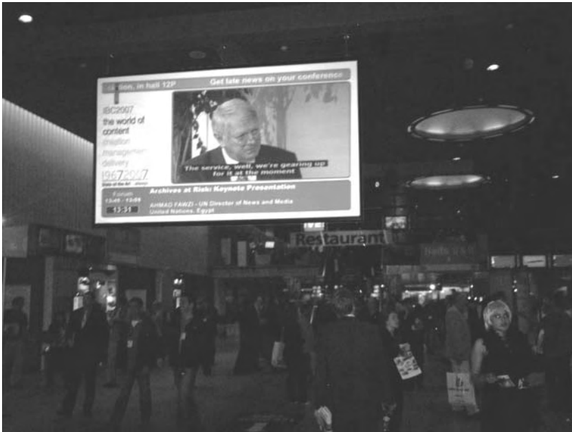
FIGURE 2.13 An Example of “Zoned” Digital Signage (Copyright 2008. Property of Jimmy Schaeffler. All rights reserved.)
