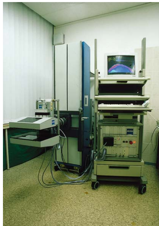
Optical Mammography. Figure 1 Prototype of a Frequency Domain optical mammograph. The instrument uses two intensity modulated (110 MHz) laser beams at wavelengths of 690 and 810 nm to scan a breast. Images are calculated from amplitude and phase data.
