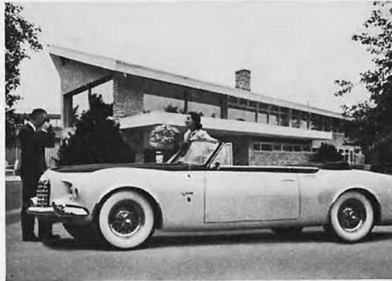
**The C-200**, designed by Chrysler and handcrafted, like the K-310, by Ghia of Turin, Italy. It is powered by the Chrysler FirePower Engine and its brakes are the new, exclusive Chrysler self-energizing disc type. The handsome chrome-plated 17" wire wheels combine lively sports car styling with practical brake-cooling design.
