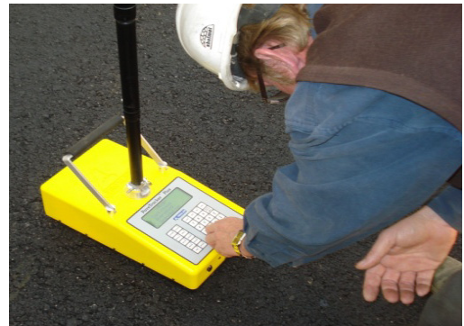
Figure 1-11. Density meter check Source: Delhi International Airport Limited (DIAL); reproduced with permission
