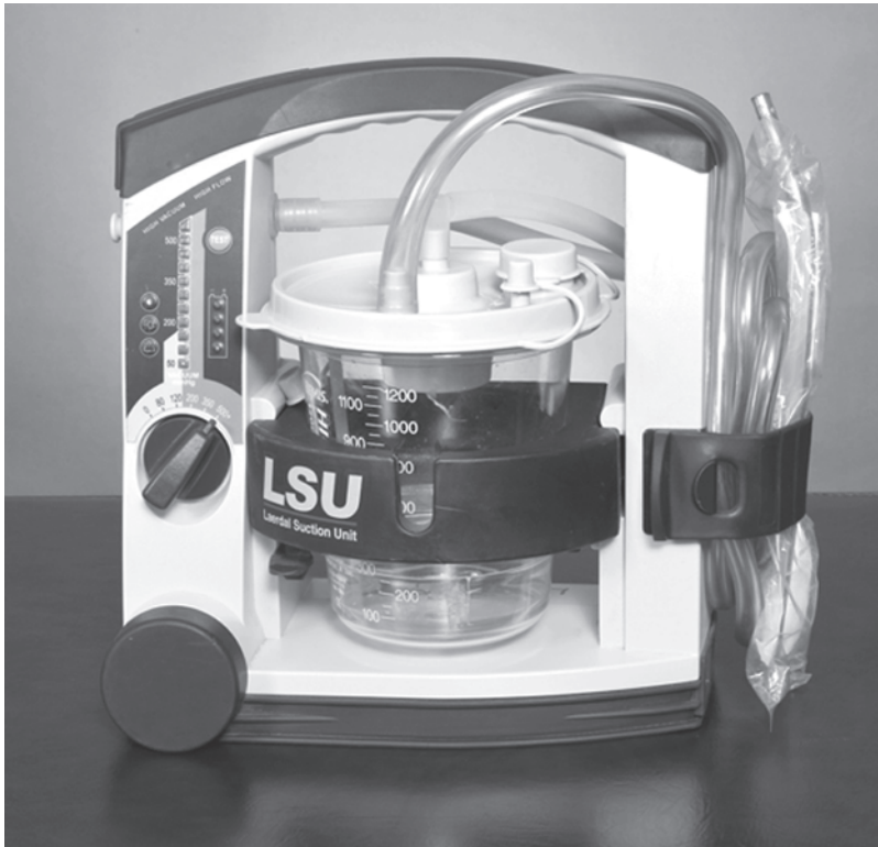
Figure 3-16. An electronic portable suction unit will clear the airway of large particulate matter but requires maintenance and regular battery charging.
