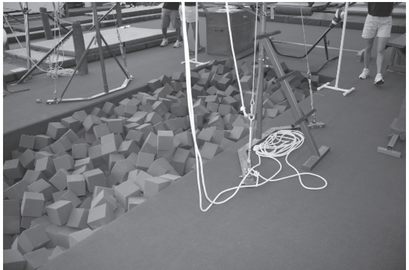
Figure 12-1. In-ground foam pit in a building designed specifically for gymnastics. Note the fixed high-bar standards on either side of the pit. This kind of equipment is considered semi-permanent because it is bolted to the floor, making it time consuming and sometimes difficult to remove.
