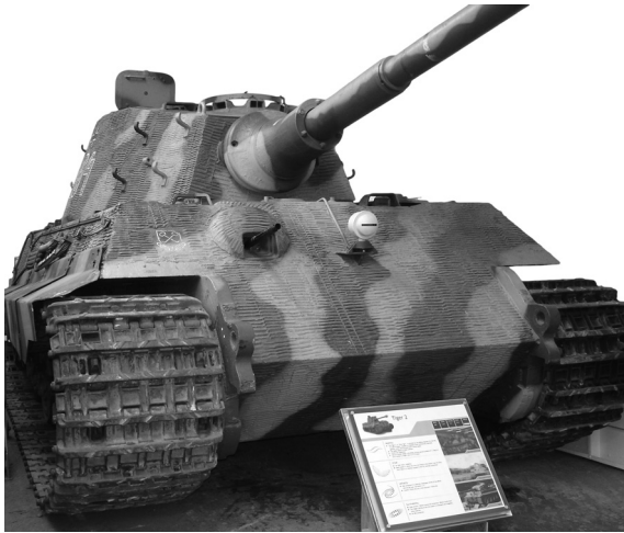
FIGURE 6.4 King Tiger tank of WWII, which used 'flame-hardened' steel armour.
