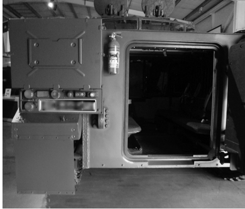
FIGURE 6.8 Rear of a Warrior IFV made from aluminium alloy plate.
