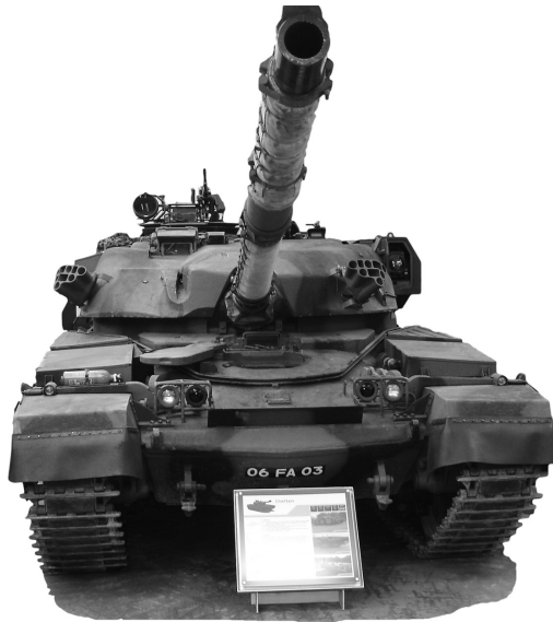
FIGURE 6.2 Chieftain Main Battle Tank (MBT) employing a cast steel turret.
