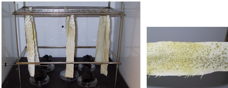
Fig. 3a (left) Test chamber at the end of test. Fig. 3b (right) Cotton strip after 30 days of incubation.
