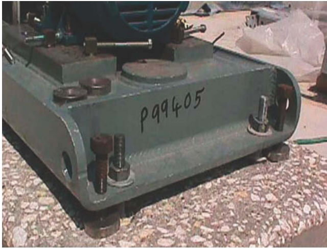
Figure 11.6 Utilizing jack pads for the jackscrew to bear against.
