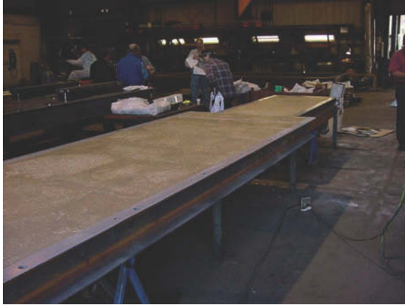
Figure 11.15 Size is not a limiting factor when it comes to pregrouting pump baseplates. However, weight may be a consideration when turning the baseplate over.
