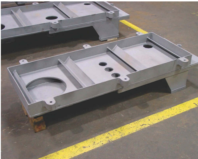
Figure 9.5 A white metal blast with a 3–5 mil surface profile gives the grout a good surface to adhere to.
