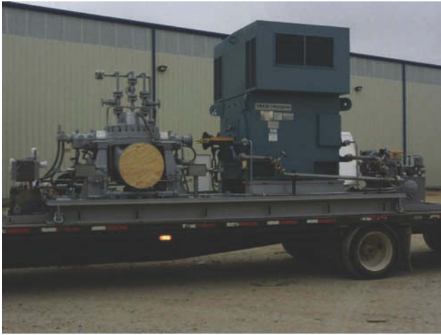
Figure 11.17 Increased rigidity offers less chance of deformation during transport.
