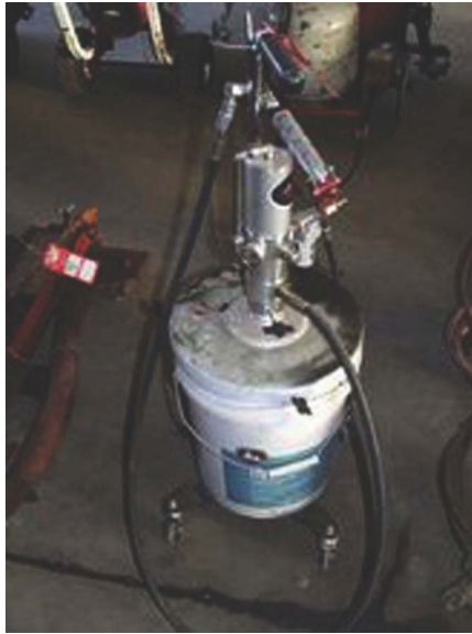
Figure 10.7 High-volume pumping system. Injection should not be greater than 30psi.
