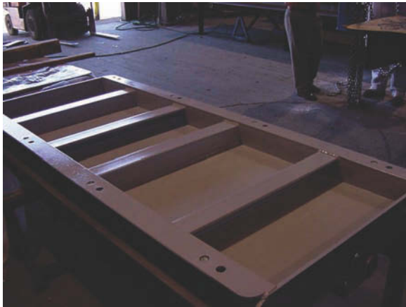
Figure 11.16 Grout holes and vent holes are not required when pregrouting a baseplate.
