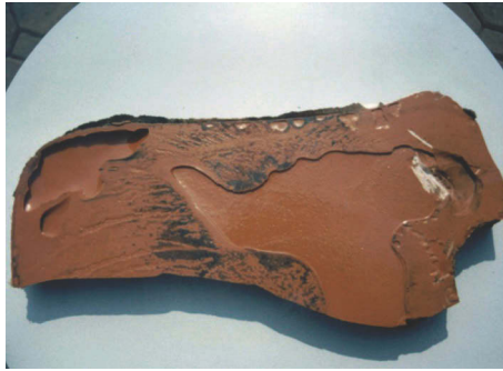
Figure 2.14 Air whipped into the grout will find its way to the surface.
