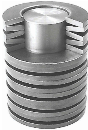
Figure 2.23 Stacking Belleville washers allow you to increase or decrease the load applied.
