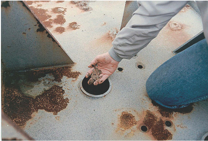
Figure 9.6 Always inspect the item to be grouted before it is set on the foundation.
