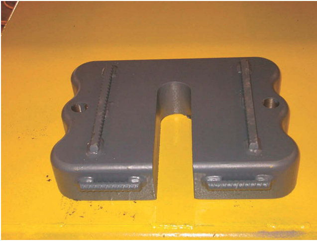
Figure 13.7 Inverted view of properly designed soleplate.
