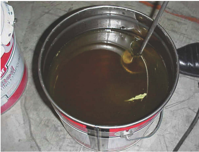
Figure 10.2 Mix completely the resin and hardener until you have a clear amber colored liquid. Do not create vortexing and whip air into the mixture.
