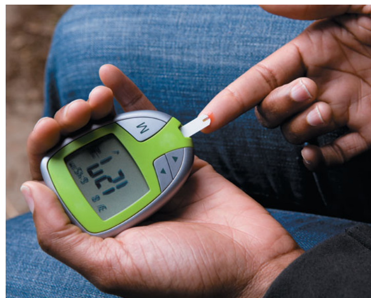
FIGURE 10a.2 A diabetic uses a glucometer to measure the amount of glucose in a drop of blood.
