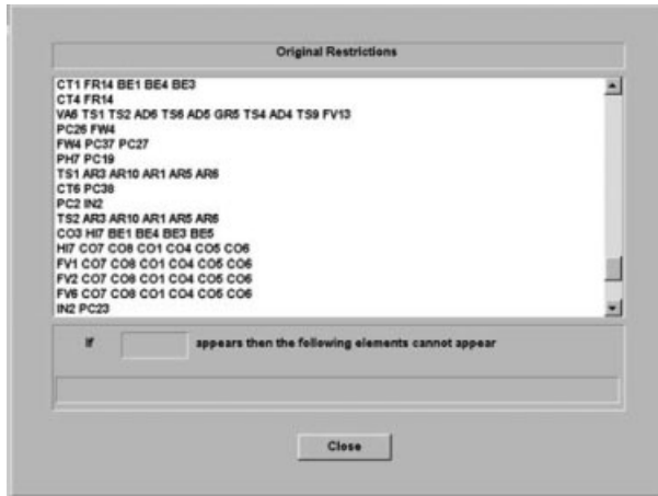
Figure 15.8. Partial set of pairwise restrictions. Each element is identified by a category code and a one- or two-digit number code showing its location within the category.
