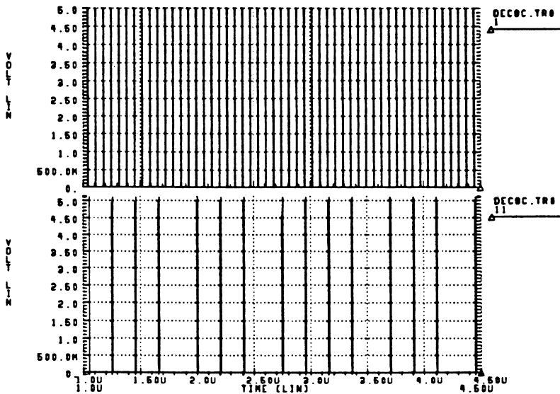
Figure 8. I/O Response of the high-pass filter at an input frequency of 14.706 MHz. The input pulse stream (top) is allowed to pass to the filter output (bottom) at a ratio of 7 output APs to 25 input APs, 28%.
