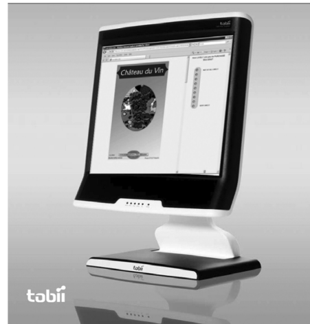
Figure 22.2 The Tobii eye-tracking device used in the project
