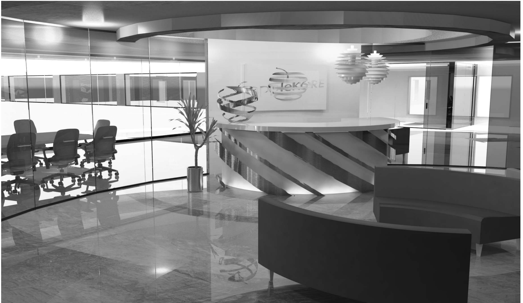
FIGURE 4-13 Perspective drawings are the most realistic looking and are often used as presentation drawings.
