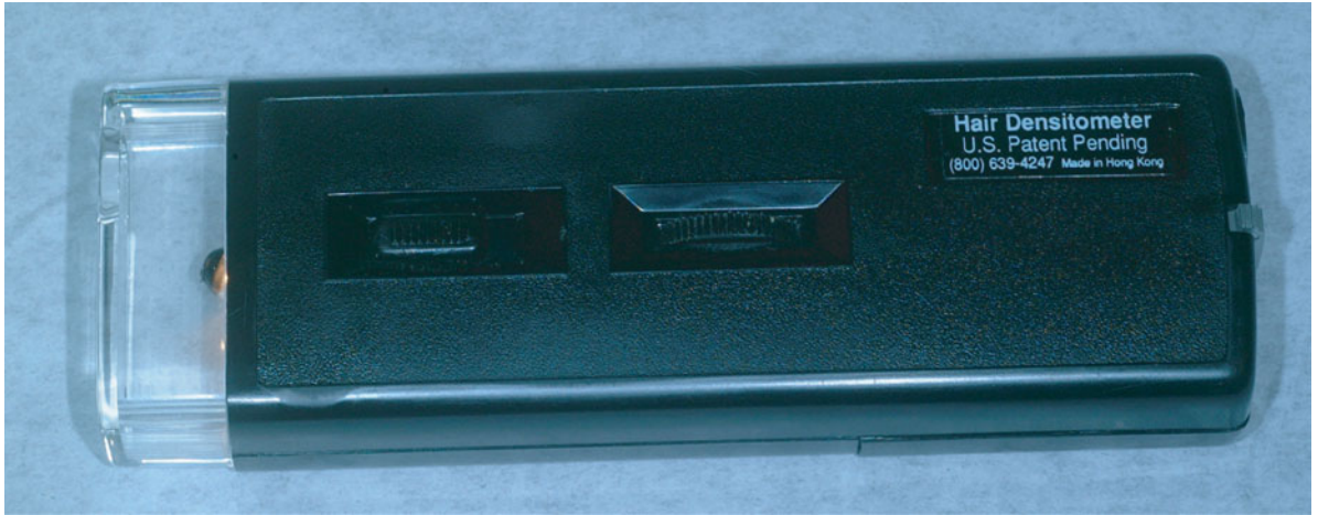
FIGURE 8.1 Portable hair densitometer may be used to calibrate donor hair density. Large caliber hair shafts greater than 70 microns yield most optimal results
