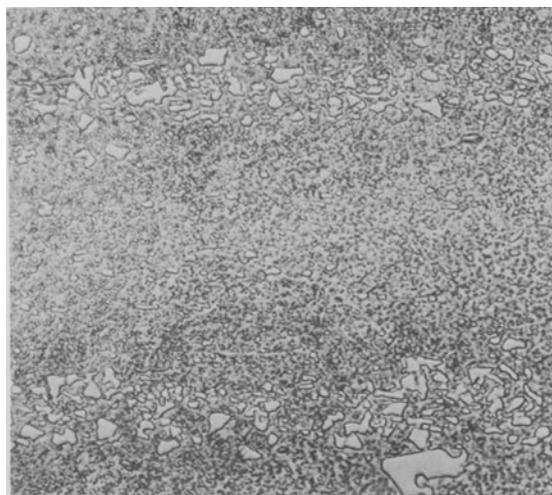
Fig. 1 Microstructure in annealed condition of specimens taken from the bar stock of heat A. Magnification 500 ×.
