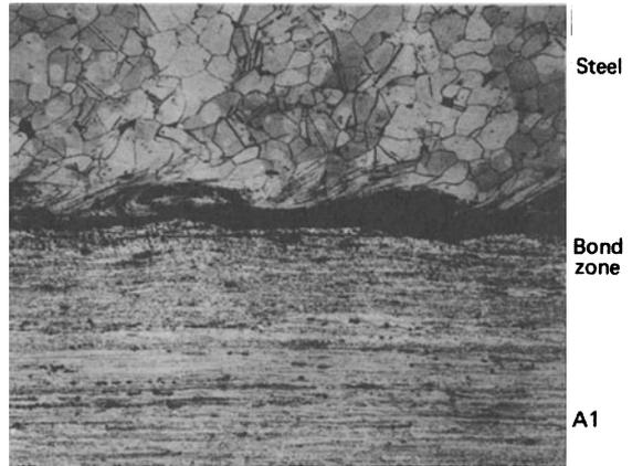
Fig. 5 Bond zone of the explosive steel-aluminium alloy-clad, 100 x.
