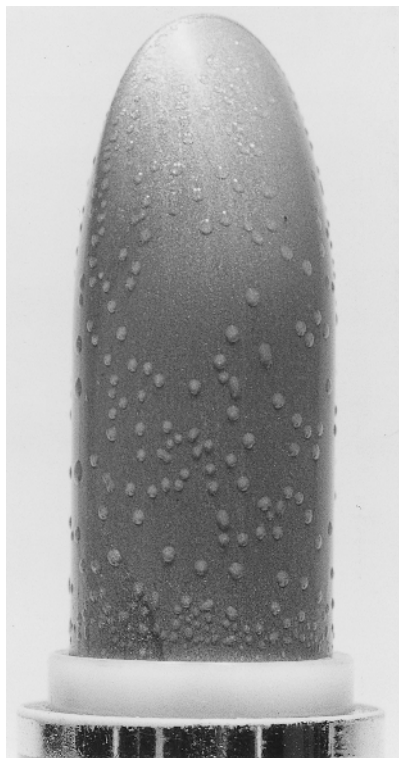
Fig. 1 Sweating on a lipstick.
