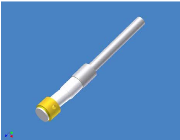
Fig. 4.9. Robot transducer mounted on a flexible head.
