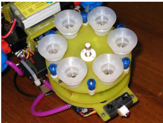
Fig. 4.8. The ultrasonic transducer mounted in the centre of the robot's foot.
