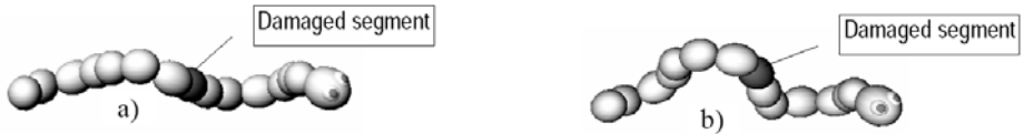
Fig. 6.16. The frontal view of the Snakebot before (a) and after the adaptation (b) to the damage of a single segment. The corresponding views from above of the sidewinding Snakebot are shown in Fig. 6.15a and b, respectively.
