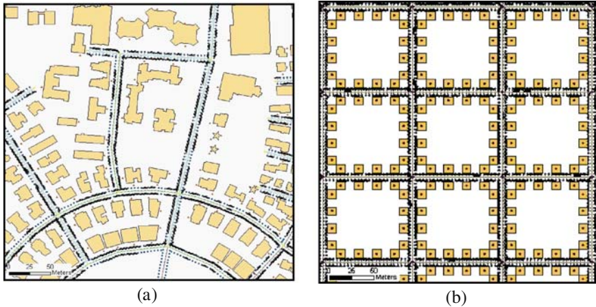
Fig. 7.1 View of the PARKAGENT map window for (a) a real city; and (b) the abstract grid network. Blue points represent road cells, small single black points represent on-street parking places and larger attached black points represent parked cars
