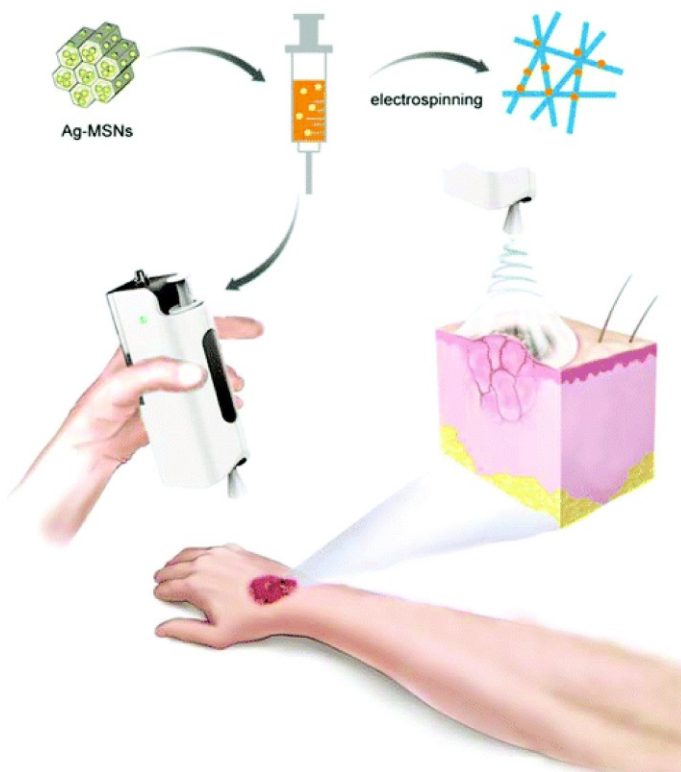
Fig. 1.21 Schematic illustration of the e-spun personalized nanofibrous dressing via a handy e-spinning device for wound healing.
