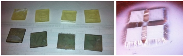
Fig. 4.7 Coated patterned collectors and electrospinning on coated collectors.
