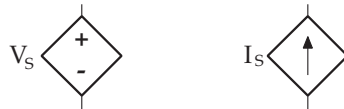
FIGURE 3.9: Basic symbols used for dependent or controlled sources. (Left) Controlled voltage source. The voltage V_s is a known function of some other voltage or current in the circuit. (Right) Controlled current source. The current I_s is a known function of some other voltage or current in the circuit.
