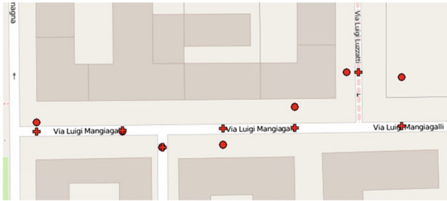
Fig. 8 Circles indicate the coordinates given by GNSS receiver, the crosses are the corrections made using as reference the nearest road segment. Note the error in the crossroads
