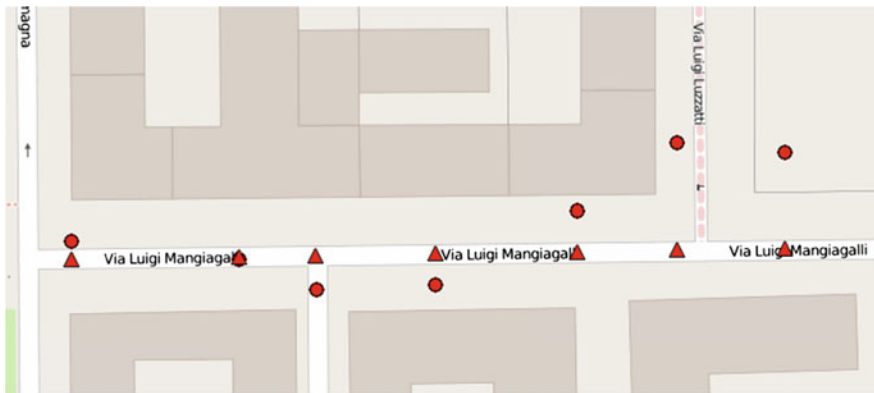
Fig. 9 Circles indicate the measured coordinates; the triangles are the correction made using as reference the nearest road segment with a bearing similar to the bearing of the movement
