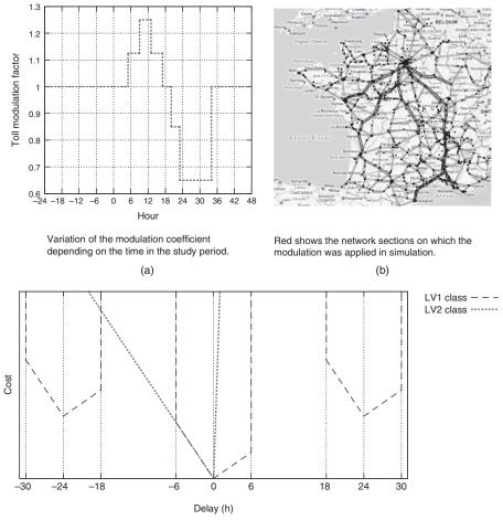
Examples of functions of cost of delay used to study price modulation with choice of departure time in the Rhone Valley.
