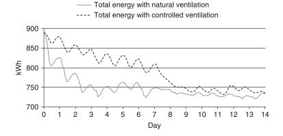
Figure 11.21 Energy in the building using a forced ventilation command and natural ventilation.
