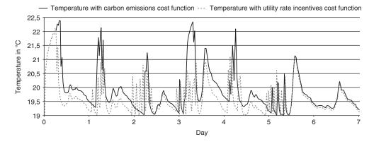
Figure 11.16 Indoor temperature for controls that flatten peak CO<sub>2</sub> emissions and the electricity consumption peak.
