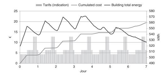
Figure 11.9 Optimal energy trajectory for one week of optimization using dynamic programming.
