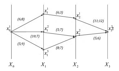
Figure 10.8 Example of sequential graph with multiple criteria. At each stage of decision  $X_i$ , different decisions (arcs of the graph) can be taken, bringing the system to a new state  $x_{i+1}^j$ . With multiple criteria, the value or performance of a decision is not a single real number but a vector of real numbers.
