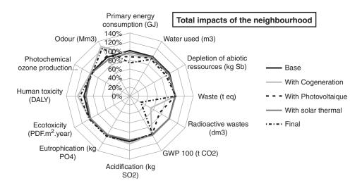
Figure 16.17 Radar chart comparing each version with the basic version.
