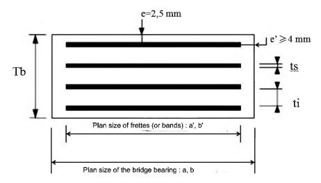
Figure 9.7 Diagram of reinforced elastomeric bridge bearings (Pirrone and Mahaffey, 2005).
