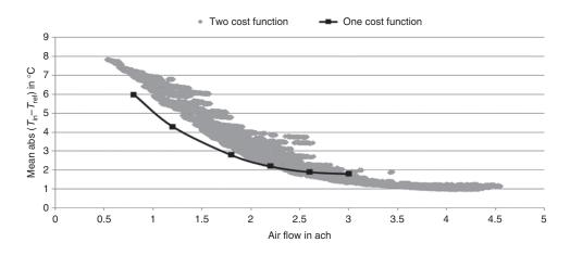
Figure 11.25 Pareto front for thermal comfort/ventilation flow.
