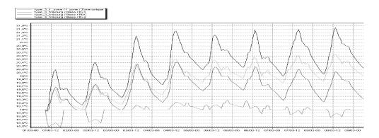
Figure 16.8 Temperature of the different floors and the single zone in mid season.
