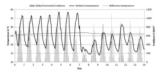
Figure 11.18 Reference temperature according to meteorology for adaptive comfort.
