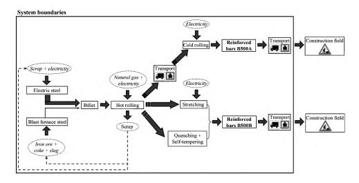
Figure 9.5 Limits of the reinforcing steel product system.
