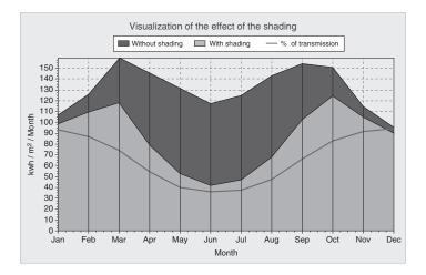
Figure 16.9 Effect of the "roof overhang" solar mask.
