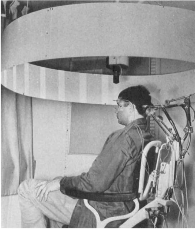
FIG. 8. The calibration test. The subject follows with his eyes as accurately as he can the moving stripes on the circular screen.
