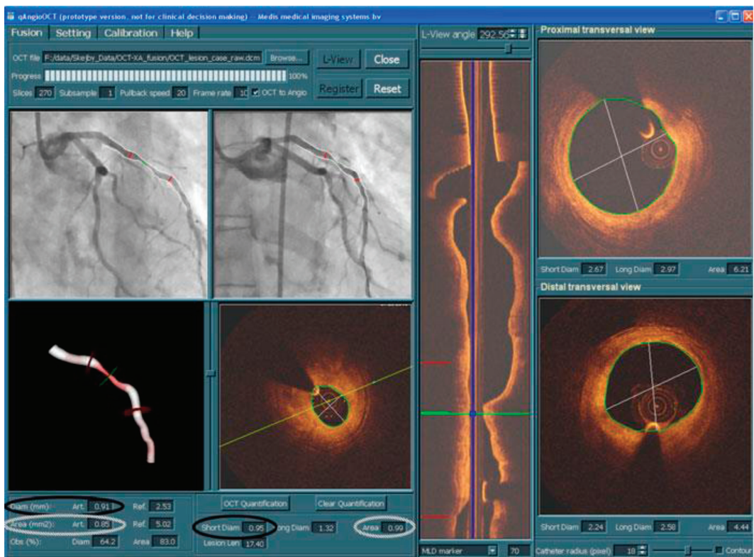
Figure 6.8 The XA-OCT coregistration and quantification. A sidebranch was manually identified from both XA and OCT images to be used as baseline position to register the two imaging modalities. After the registration, the markers superimposed in the OCT longitudinal view were synchronized with the same markers in the XA views. The OCT measurements could be compared with 3D QCA at the same position. (From Tu S et al., Int J Cardiovasc Imaging , 27, 197–207, 2011. With permission.)
