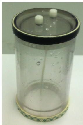
Figure 3.5 The specially designed cylindrical shell phantom can be fit inside the SPECT insert and is used in uniformity correction of the detector pixels. The precisely machined thin cylindrical shell is filled with radioactive solution to provide a uniformity image of all the pixels of the cylindrical detector ring of the SPECT insert for nonuniformity correction.
