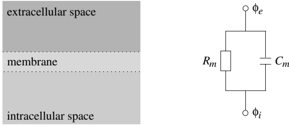
Fig. 7.4. Cell membrane and its approximation by resistor-capacitor circuit. The circuit consists of a nonlinear resistor R_m and a capacitor C_m . The voltage over the membrane V_m is hereby defined as the difference between the extracellular potential \phi_e and the intracellular potential \phi_i
