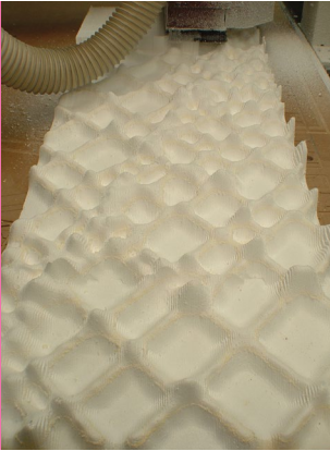
FROM LEFT: Milled-foam substrate; panels of milled-foam substrate; laying fiberglass over milled-foam substrate. BELOW: Underside of canopy. OPPOSITE: Assembled canopy.
