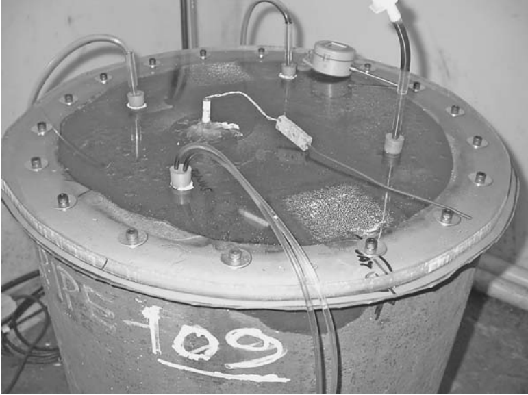
FIGURE 11.30 24-in diameter full-ring test as per OTI 95-635 containing 300 L of NACE TM0177-96 solution saturated with H_2S . (Courtesy of Bodycote Materials Testing)
