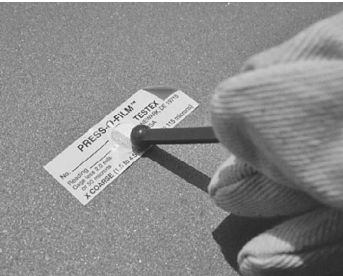
FIGURE 14.23 Burnishing Testex Press-O-Film replica tape. (Courtesy of KTA-Tator, Inc.)
