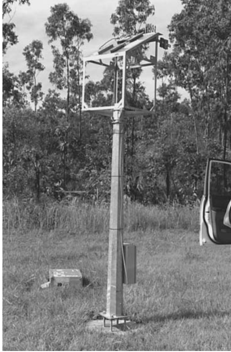
FIGURE 9.41 Outdoor exposure test station with specimen rack on top and data logger attached below at an army base in Northern Australia. (Courtesy of DSTO Australia)
