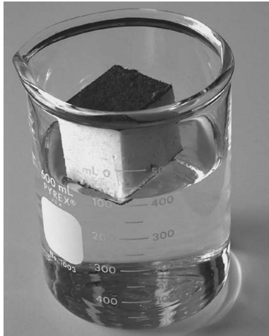
FIGURE 6.27 Sample of isocyanurate foam still floating on water after six weeks.
