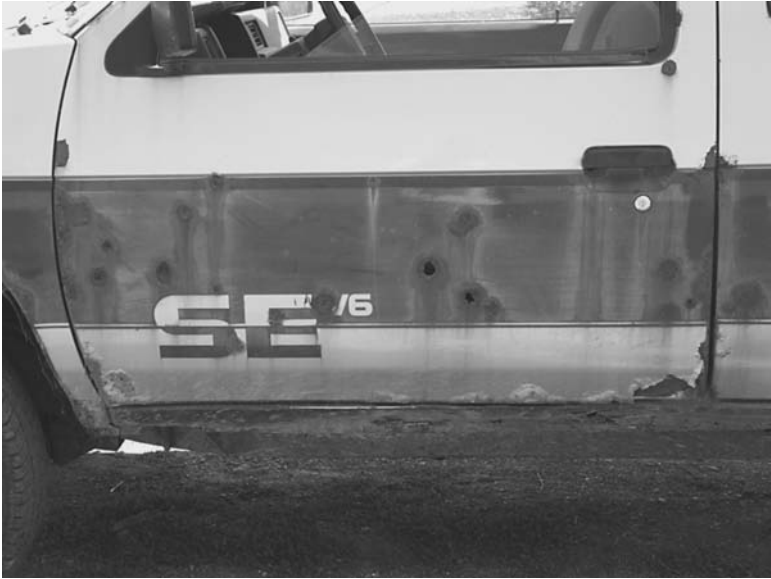
FIGURE 9.14 A truck all corroded on the driver side due to salt on the road.
