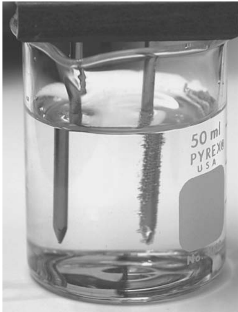
FIGURE 7.30 Experiments to illustrate the effects of stray current showing (a) the experimental setup containing a DC power supply plus two steel nails partially immersed in a dilute saline solution and connected to the positive (left) and negative (right) posts of the DC supply; the effects of imposing a DC current on the nails (b) after five and (c) ten minutes.
