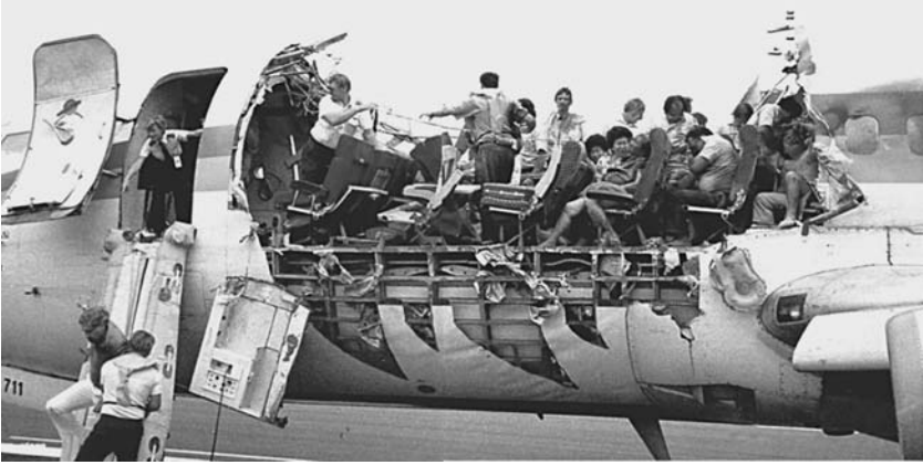
FIGURE 7.33 Photograph of the Boeing 737 operated by Aloha Airlines that lost a major portion of the upper fuselage in 1988.
