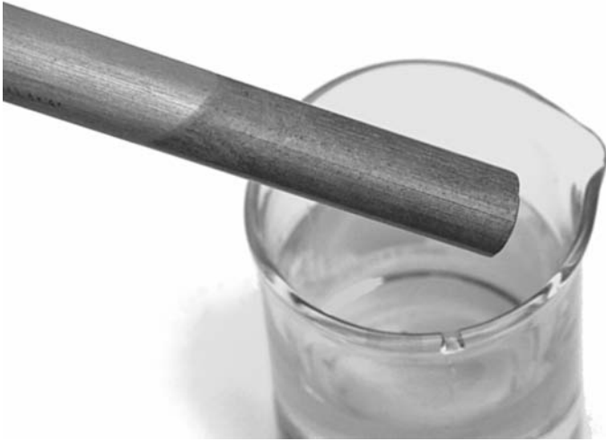
FIGURE 6.34 Plating out of copper nodules on an aluminum rod immersed in a 0.2 M copper sulfate solution.
