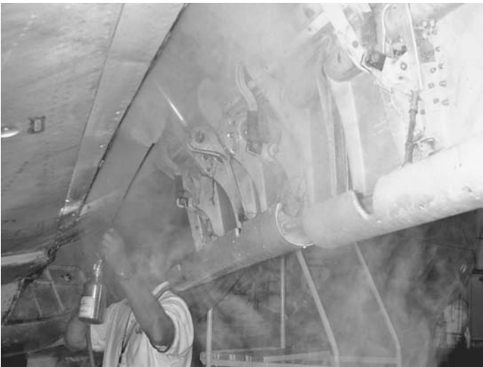
FIGURE 14.7 Fogging of aircraft with a commercial CPC.
