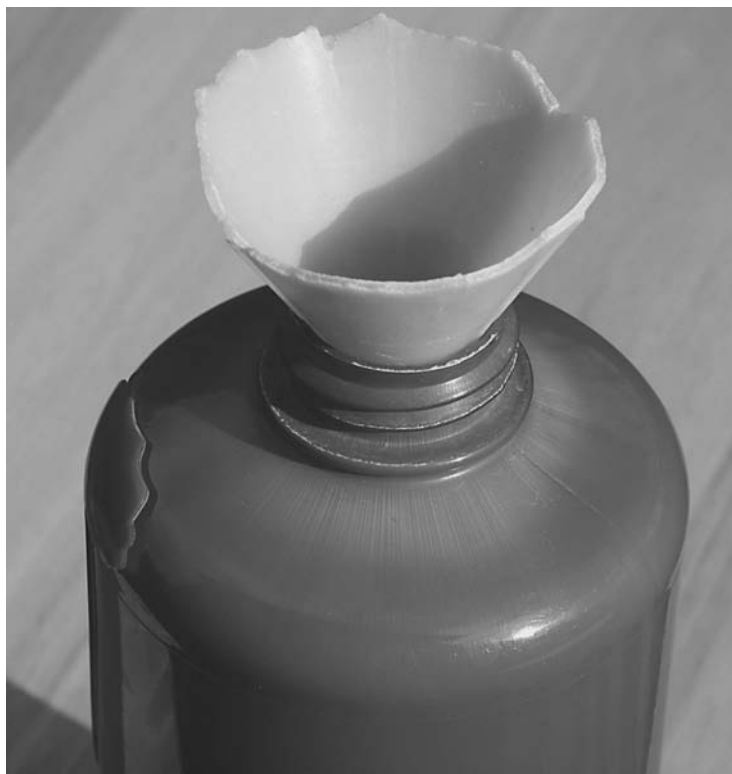
FIGURE 9.52 Polycarbonate (Nalgene) bottle and polypropylene funnel degraded over a few years of exposure to sun rays on a window sill.
