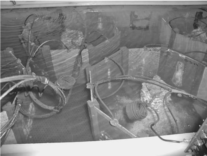
FIGURE 14.30 Laboratory setup to test for disbonding during the application of cathodic protection. (Courtesy of Corrpro)
