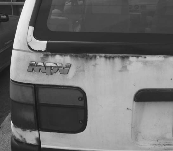
FIGURE 6.24 Sand trapped behind trim can wear away the protective paint coating and expose the steel to the environment and subsequent severe corrosion damage.
