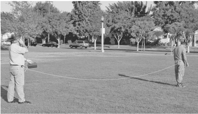
FIGURE 13.39 Pipeline CP fault testing with Pearson-type detector. (Photo courtesy of Tinker & Rasor)
