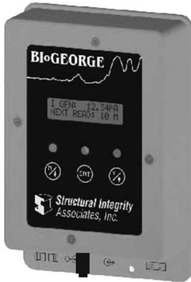
FIGURE 10.15 Control box of a BioGEORGE MIC detection probe. (Courtesy of George Licina, Structural Integrity Associates, Inc)
