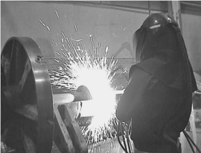
FIGURE 14.14 Arc-spraying process. (Courtesy of M. Gariepy, WEIR Engineering Services, Montreal, Canada)
