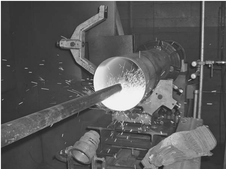
FIGURE 14.16 Plasma-blowing torch for metallizing inside pipes and tubes. (Courtesy of M. Garipey, WEIR Engineering Services, Montreal, Canada)
