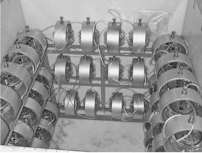
FIGURE 11.28 Bank of 50 NACE TM0177 method, a constant strain test facility with uniaxially loaded tensile specimens. (Courtesy of Bodycote Materials Testing)
