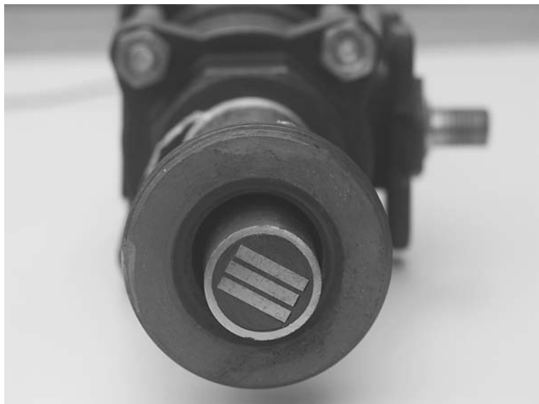
FIGURE 5.33 Close-up of corrosion sensing elements used for thin film corrosion monitoring. (Courtesy of Kingston Technical Software)
