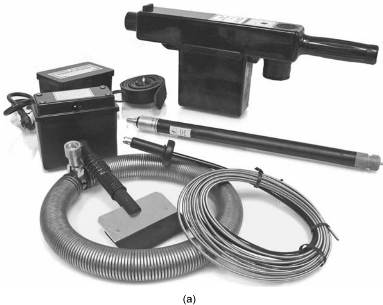
FIGURE 14.31 High voltage holiday detector kit (a); low-voltage holiday detector (b); holiday testing with high voltage detector (c). (Courtesy of Tinker & Rasor)
