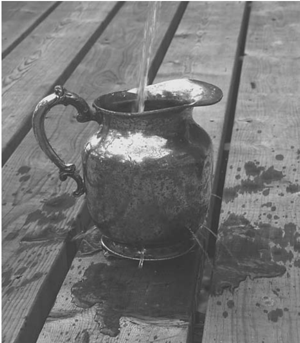
FIGURE 6.8 Water freely flowing out of a silver-plated water jug with pit through corrosion.
