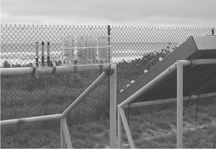
FIGURE 9.32 Metal coupons in a plastic test rack exposed at the Kennedy Space Center beach corrosion test site besides a CLIMAT coupon. (Courtesy of Battelle)
