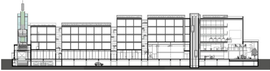
Fig. 12.12 Longitudinal section over the EVA Centre with integrated Sustainable Implant, SI (left) and Living Machine integrated in the entrance area (right)
