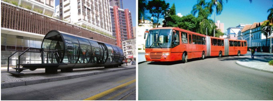
Fig. 12.15 The recognisable bus stops ( left ) in the city (similar to above-ground tube stations –without thresholds between bus and platform) and large fast-lane buses ( right )
