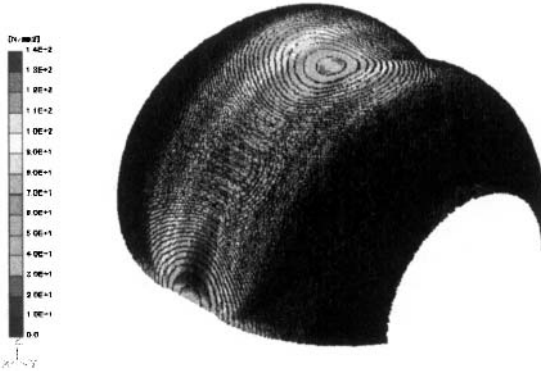
Fig. 6 Thermal deformation and stress distribution of a thin half spherical shell with circular cutting defined in 256 x 256 x 256 grid space computed by 3D-HMG.
