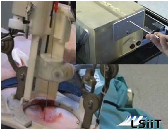
Fig. 5 Teleoperated needle insertion experiment
