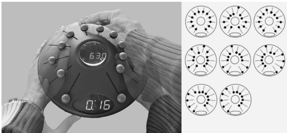
Figure 21.4 Setting the sliders of the working prototype for Wensveen's (Wensveen et al. 2002) alarm clock (left) and different final slider settings of expressive behaviours (right)
