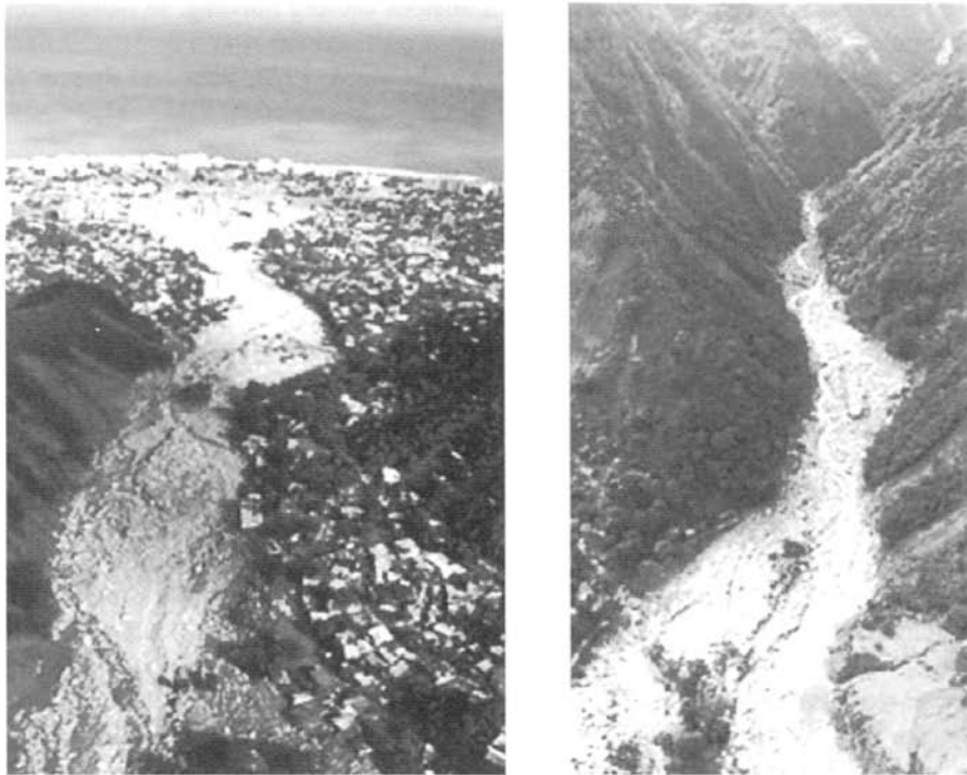
Figure 1 (see color insert) Quebrada San Julián upstream of Caraballeda showing evidence of recent debris flows and flash floods. Note the high slope angles, large numbers of debris flow scars, and abundance of new alluvium and colluvium in the channel bed and fan surface. See ftp site for color image.
