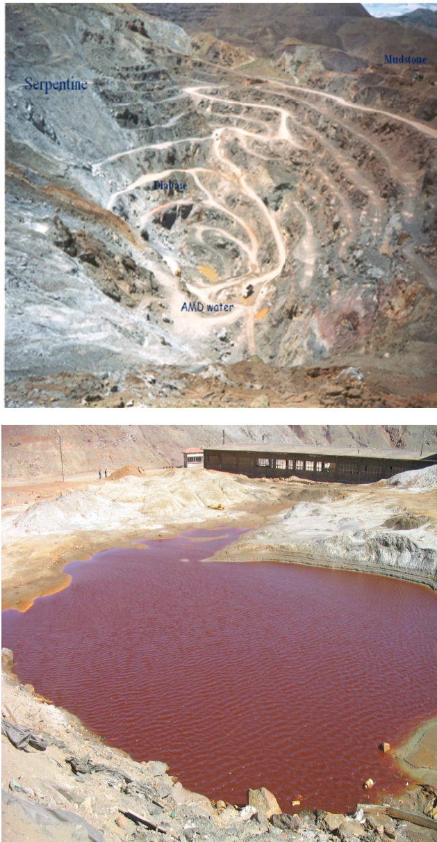
Fig. 4. AMD waters in the Maden copper deposit.
