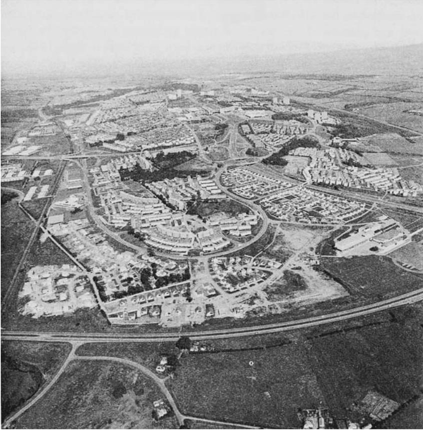
**Plate 6.4** (b) Milton Keynes new city, Buckinghamshire. Designed in the late 1960s, this is planned as a series of low-density housing areas in the interstices of a rectangular highway grid. The aim is to promote easy mobility both by private car and by public transport. It has been more successful in the former than the latter.
