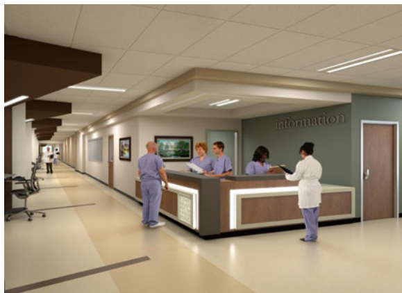
Fig. 4.50 Parkland Hospital Dallas, USA—Inpatient units feature decentralised caregiver workstations between every two patient rooms thereby providing visual access into each room, which increases observation capabilities and allows for a higher level of care. (Source HDR + Corgan 2012)
