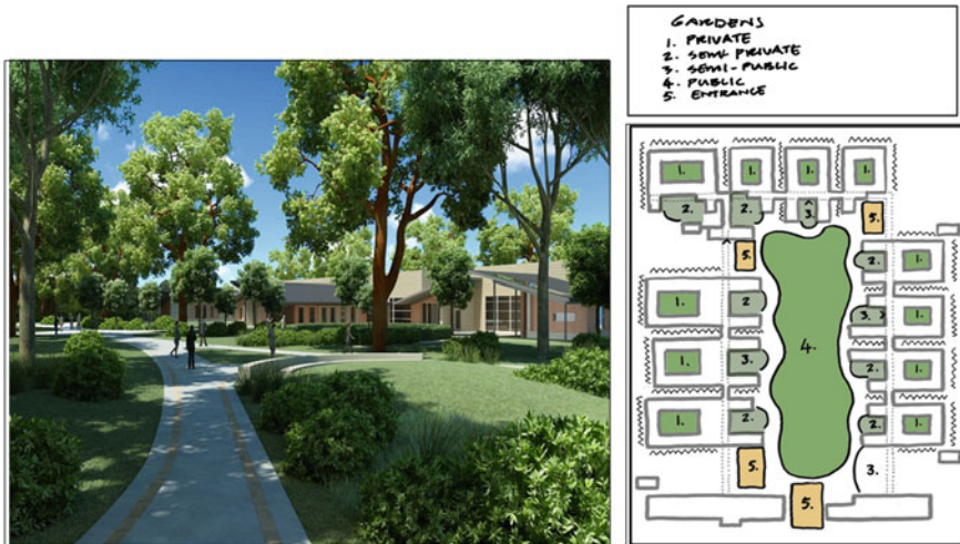
Fig. 4.85 Glenside Campus Redevelopment Australia—‘Village-like’ configuration around a shared garden: The gardens are designed to indicate a hierarchical progression from public, semi-public, semi-private to private gardens (Source Swanbury Penglase Architects 2012)
