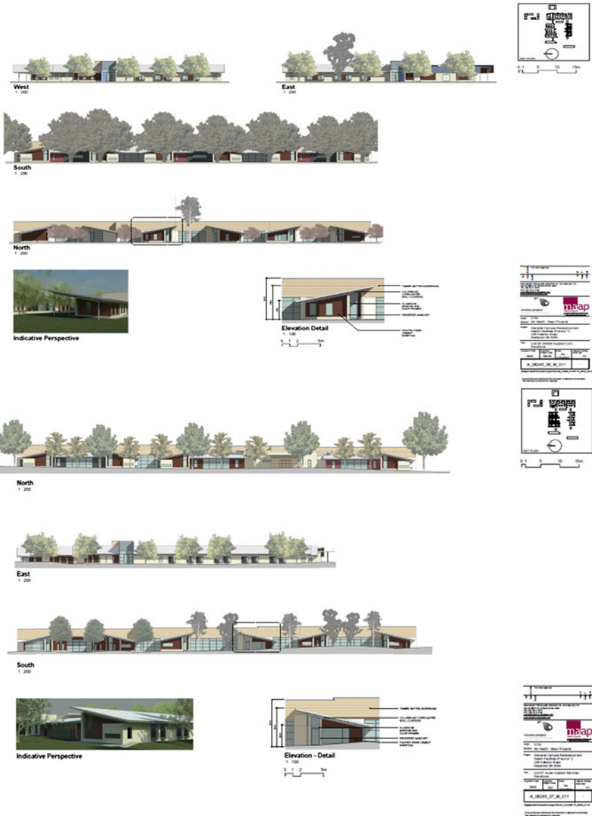
Fig. 4.111 Glenside Campus Redevelopment Australia—Elevations 2: To overcome the social stigma or de-stigmatise the existing site and its Victorian Asylum references courtyard buildings of a domestic scale arranged around a shared central “healing garden” which is then accessible to both patients and the public alike are provided (Source Swanbury Penglas Architects 2012)
