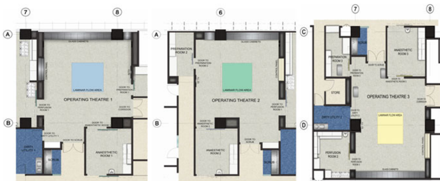
Fig. 4.125 National Heart Centre, Singapore—Operating theatres 4: floor layout plans for the 3 theatres—Integrating advances in medical technology within the operating theatre environment (Source Broadway Malayan Singapore 2012)
