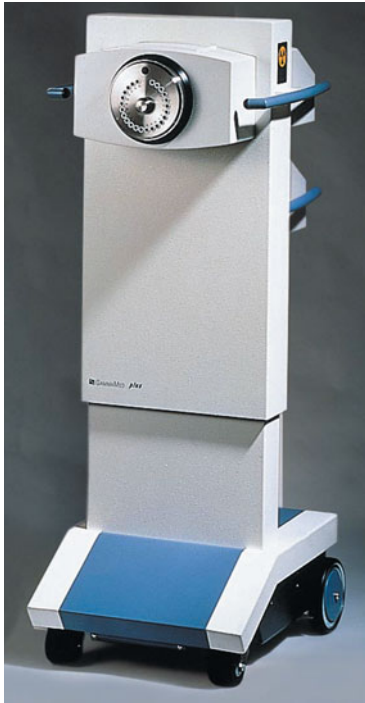
Figure 5.2 A modern brachytherapy afterloading machine, which uses a small iridium source located in the head of the machine that passes out by remote control through a series of channels to deliver radiation into applicators within a tumour area connected to these outlets. (Courtesy of Varian Medical Systems)
