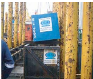
Result of stacking of basket with imbalanced load
