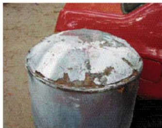
Bulging of the bottom of the drum after the explosion
