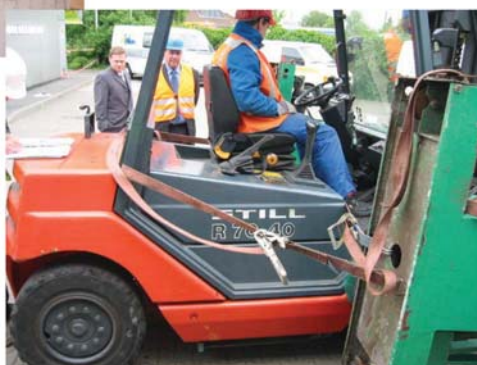
Reconstruction of the incident. The retaining strap passes behind the driver's heels
