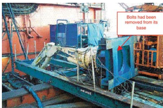
Toppled SIMOPS crane
