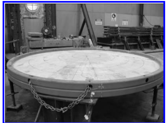
Figure 2. Shallow dome tested to failure.
