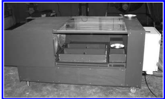
Figure 1. Climate chamber showing two rectangular moulds and one square mould for concrete as well as one pan for water.
