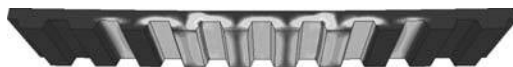
Figure 1. Contours of scaled damage measure in concrete fill due to cracking caused by sagging moments.
