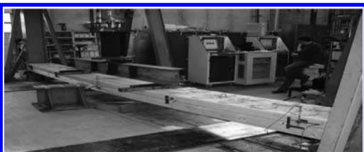
Figure 1. Test set up for dynamic and static tests of timber – concrete slabs.
