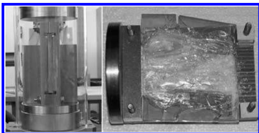
Figures 2a and 2b. Testing facility for block materials and failed glazing with aluminium blocks.
